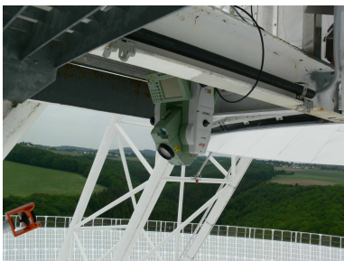
Figure 3. Leica TCRP 1201, mounted top-down.
