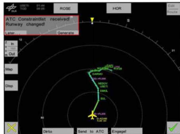
Fig. 4: The AHMI, a graphical user interface supporting interaction between AFMS and pilots
