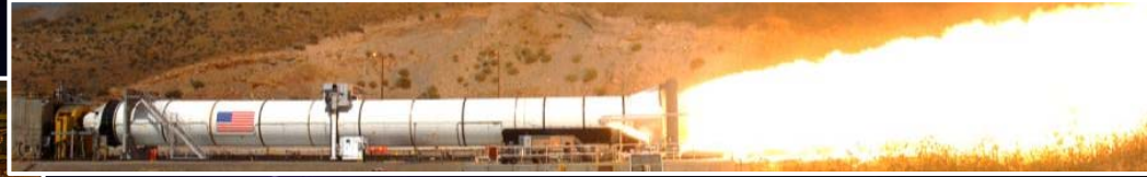
Solid Rocket Booster development motor test, Promontory, Utah, Sep 2011.
