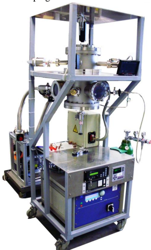
Fig. 4 (left): UHV Chamber with oscillating quartz crystal for mass loss/evaporation rate determination
