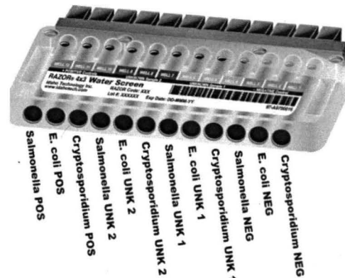
Figure 1. RAZOR EX water processing pouch. Each pouch contains 3 targets ( Cryptosporidium , Salmonella , and Escherichia coli ) that are relevant to water systems monitoring. For this evaluation, the food pouch that detects Campylobacter , Listeria monocytogenes , and Salmonella was also utilized. Image from BioFire Diagnostics website: http://www.biofiredx.com/RAZOREX/index.html .
