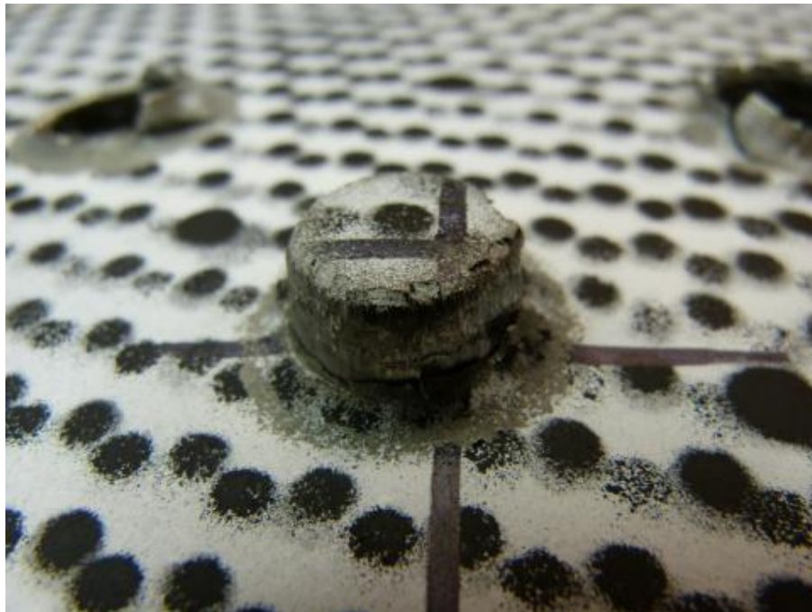
Figure 22.—Example of plug formed in 0.5 in. Ti-6Al-4V plate.
