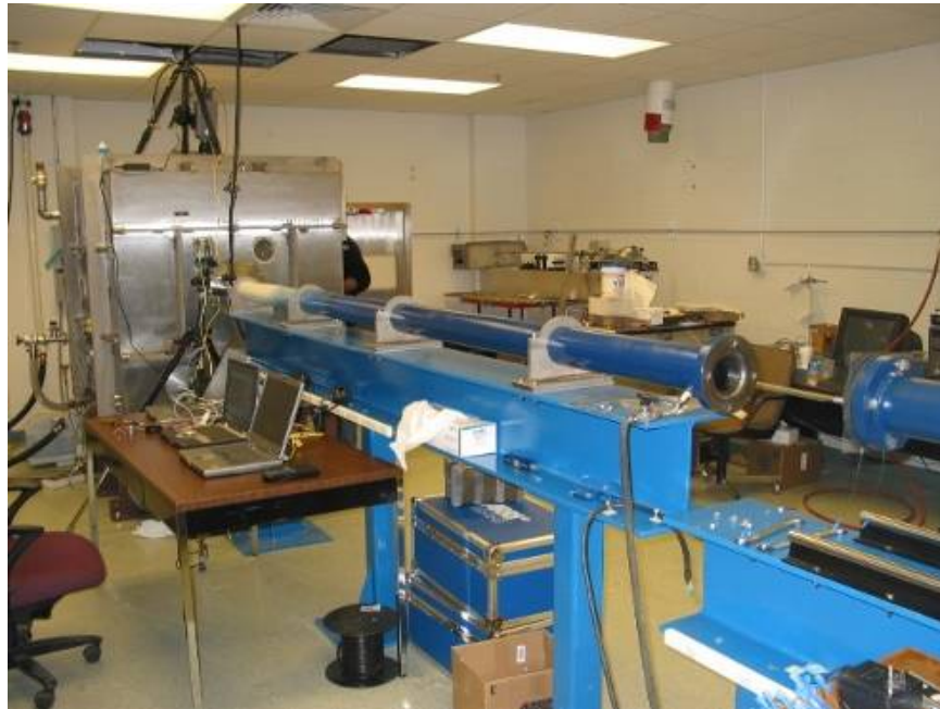
Figure 4.—Large Vacuum Gas Gun (shown with 3 in. diameter gun barrel).
