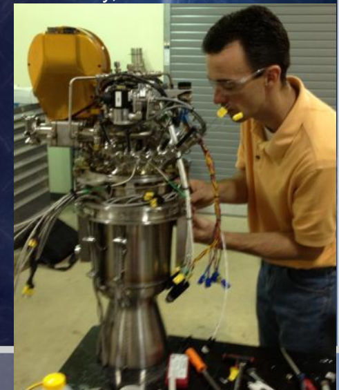
HD5: Yr2012-2013, 67 tests at SSC, >160 sec total run time. Instability, thermal issues.
