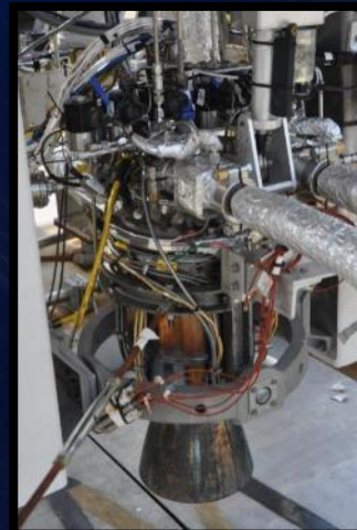
Yr2012-2013, rebuilt as HD4-LT (large throat), 36 starts (incl. 12 vehicle tests), 285 sec total run time, current Morpheus engine
