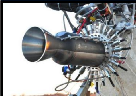
HD3: Yr2011, 27 tests (incl. 8 vehicle tests), 363 sec total run time, burnthrough-damaged
