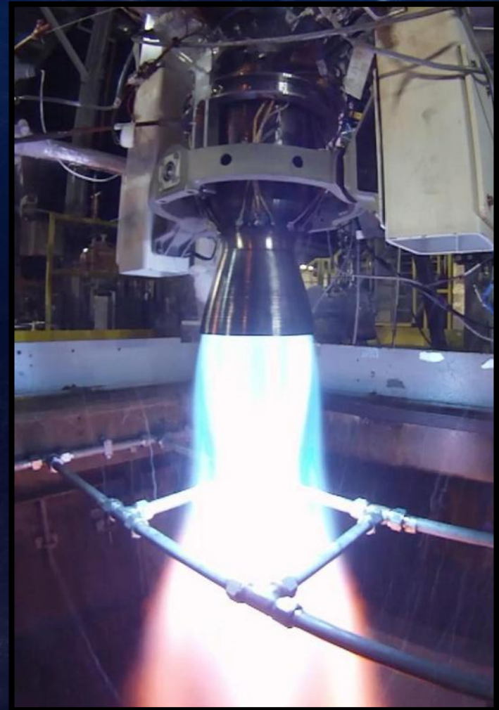
HD5 installed in SSC stand E-3
