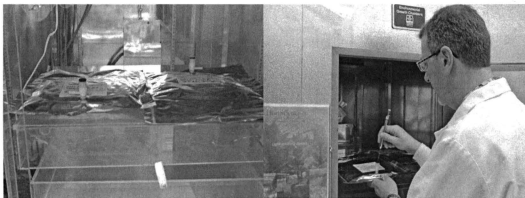
Figure 3. Storage bags used to store HMC prepared tiles. Picture A shows the bags inside the chamber. B shows samples being taken for gas analysis.
