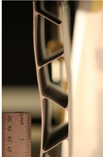
Figure 15. Buckling of a fluted core sample.
