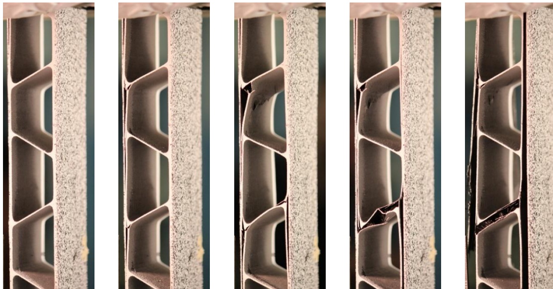
Figure 10. Fluted core tension test, damage propagation.
