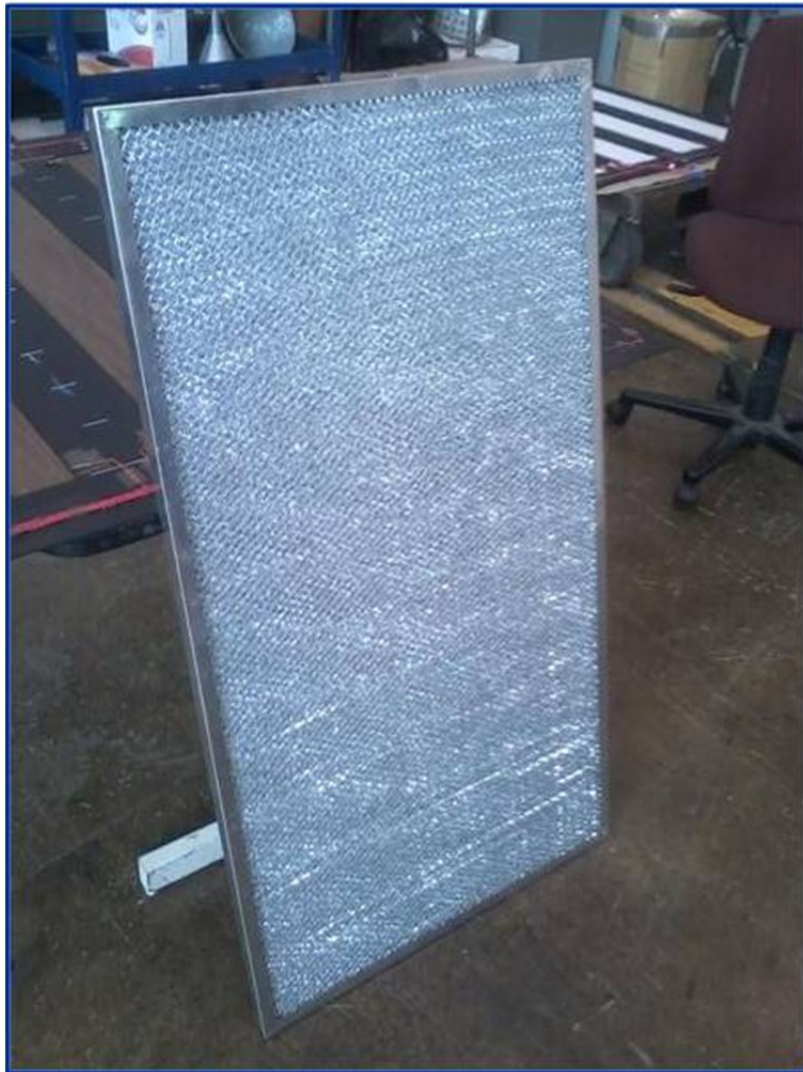
Figure 8.—Photo of one of two aluminum mesh heat exchanger panels (L2).
