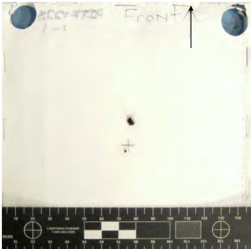
Figure 88 Overall View of Damage to Front of MLI (scale in 5mm increments / black arrow indicates flight path of projectile)
