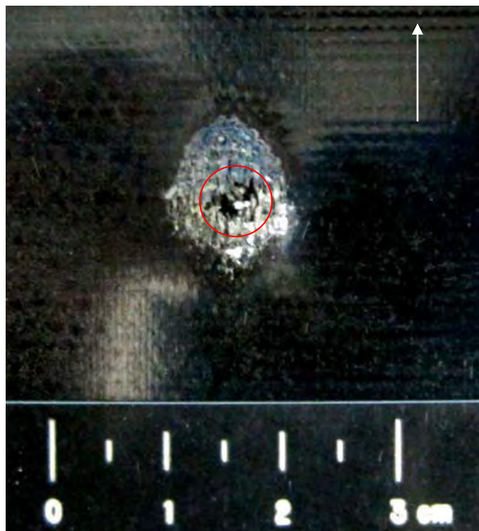
Figure 114 Close-up View of Damage to Back Side of NP 504 Substrate (scale in 5mm increments / white arrow indicates flight path of projectile)
