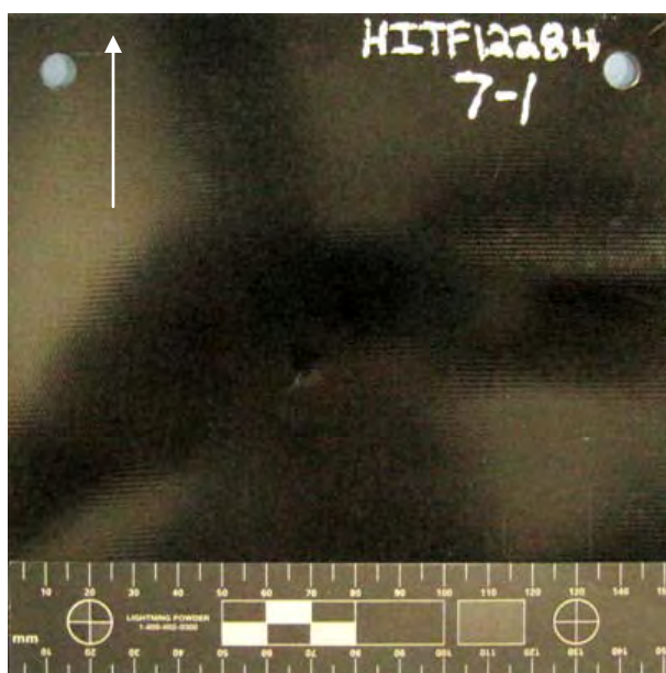
Figure 30 Overall View of Damage to Back Side of NP 504 Substrate (scale in 5mm increments / white arrow indicates flight path of projectile)
