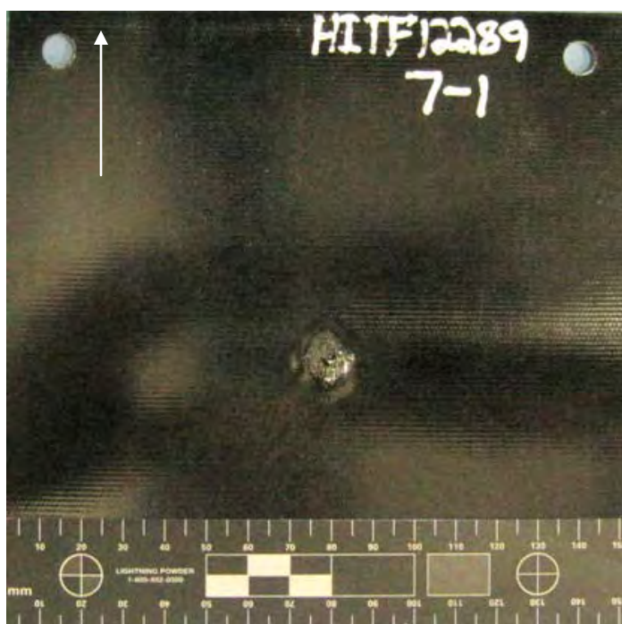
Figure 113 Overall View of Damage to Back Side of NP 504 Substrate (scale in 5mm increments / white arrow indicates flight path of projectile)
