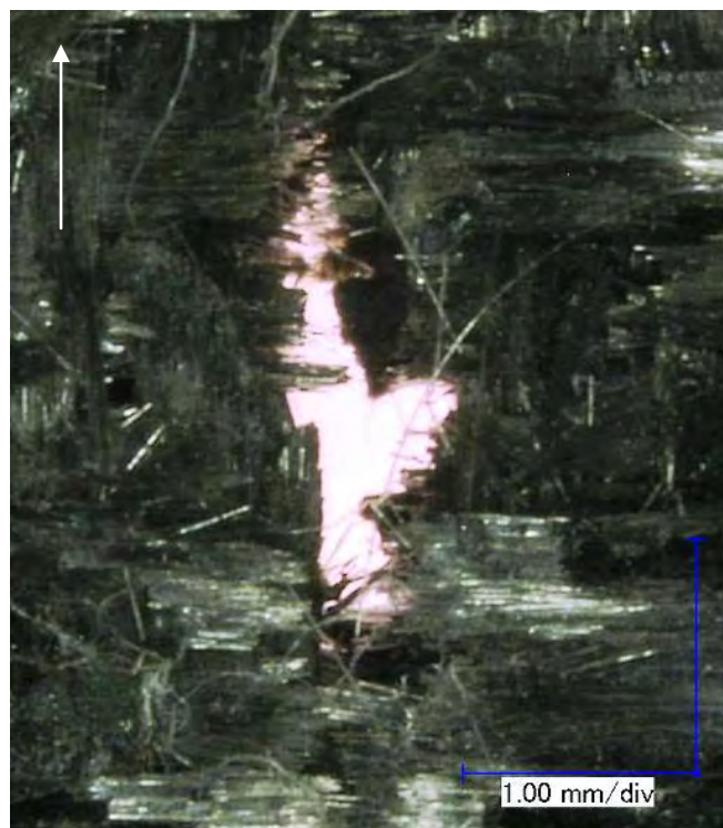
Figure 448 Close-up View of Most Significant Damage to Back Side of NP 504 Substrate (black arrow indicates flight path of projectile / damage within red circle in Figure 472)
