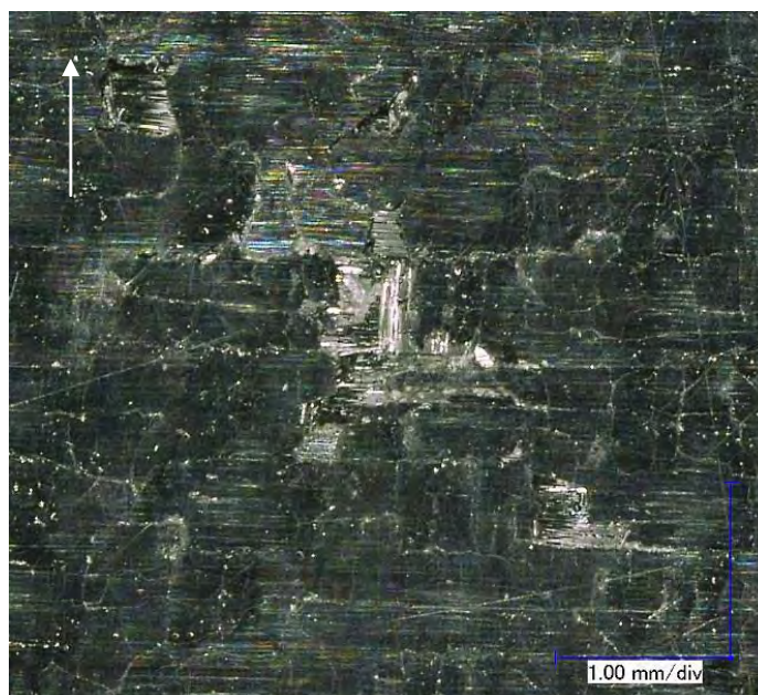
Figure 274 Close-up View of Most Significant Damage to Back Side of NP 504 Substrate (white arrow indicates flight path of projectile / damage within red circle in Figure 273)
