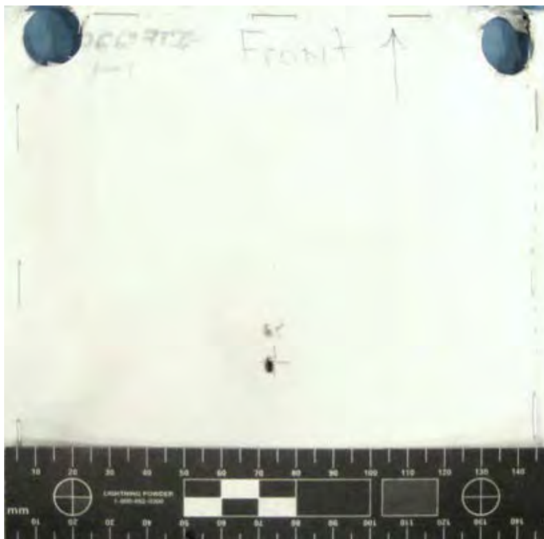
Figure 266 Overall View of Damage to Front of MLI (scale in 5mm increments / black arrow indicates flight path of projectile)
