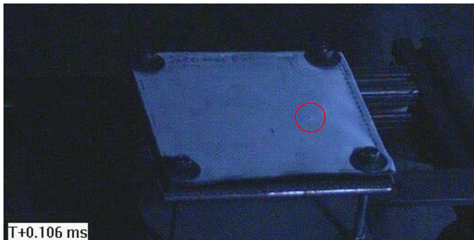
Figure C13 Image of Projectile Captured Prior to Impact (via Phantom v711 / projectile within red circle)
