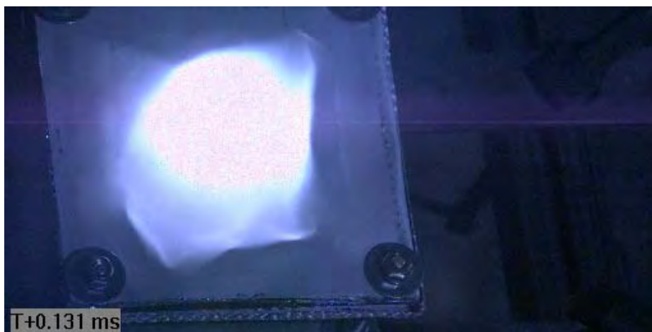
Figure C32 Projectile Impacting Target (via Phantom v711)
