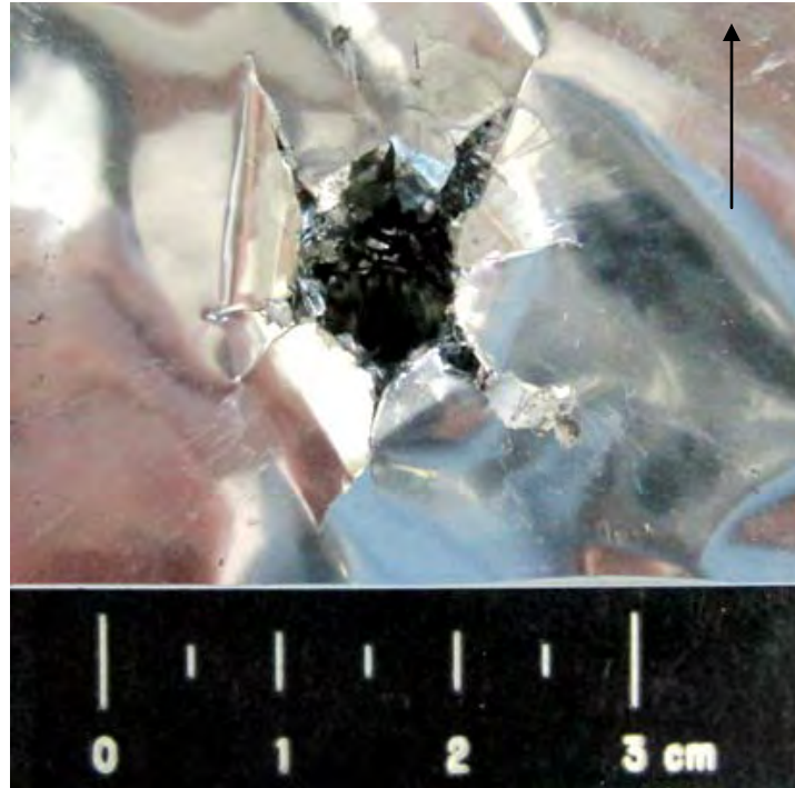
Figure 42 Close-up View of Damage to Back Side of MLI (scale in 5mm increments / black arrow indicates flight path of projectile)
