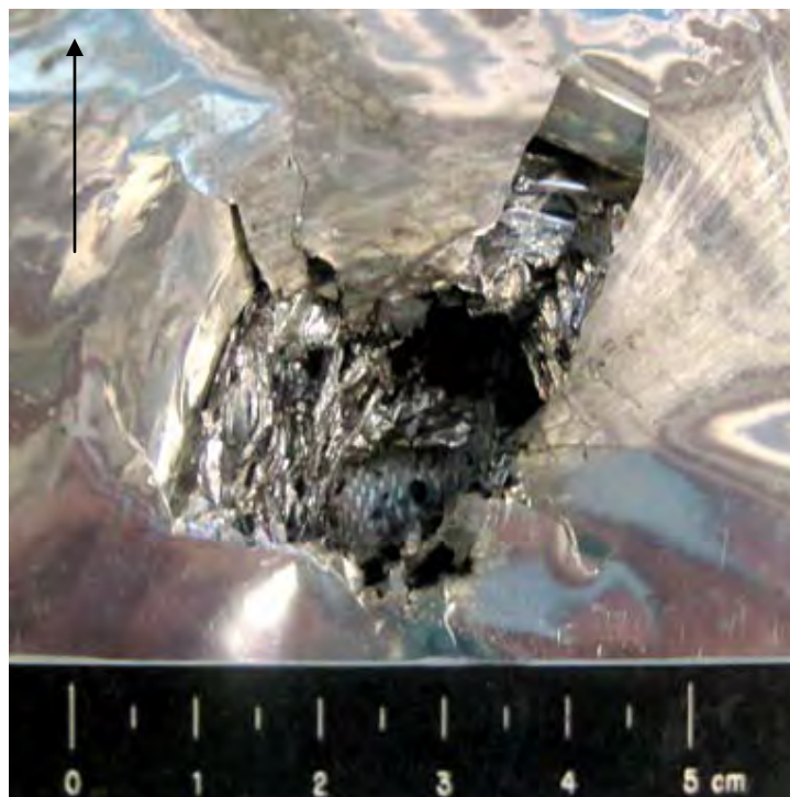
Figure 443 Close-up View of Damage to Back Side of MLI (scale in 5mm increments / black arrow indicates flight path of projectile)
