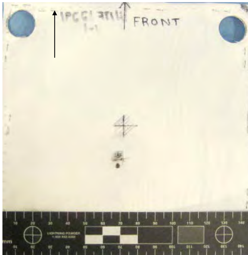
Figure 140 Overall View of Damage to Front of MLI (scale in 5mm increments / black arrow indicates flight path of projectile)
