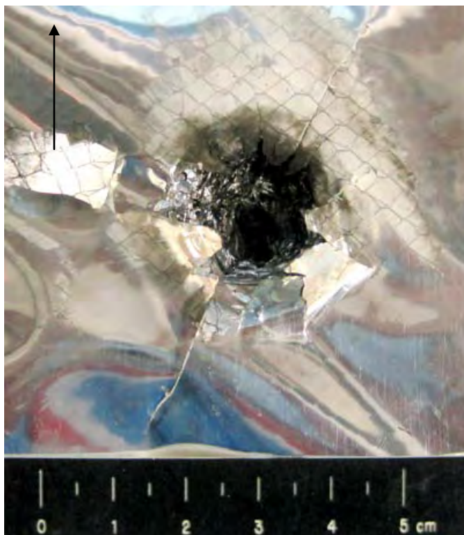
Figure 218 Close-up View of Damage to Back Side of MLI (scale in 5mm increments / black arrow indicates flight path of projectile)
