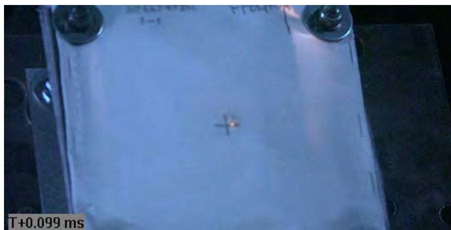
Figure C3 Projectile Impacting Target (via Phantom v711)
