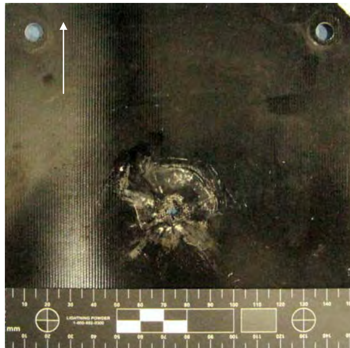
Figure 343 Overall View of Damage to Front of NP 504 Substrate (scale in 5mm increments / white arrow indicates flight path of projectile)
