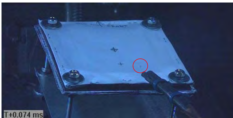
Figure C34 Image of Projectile Captured Prior to Impact (via Phantom v711 / projectile within red circle)
