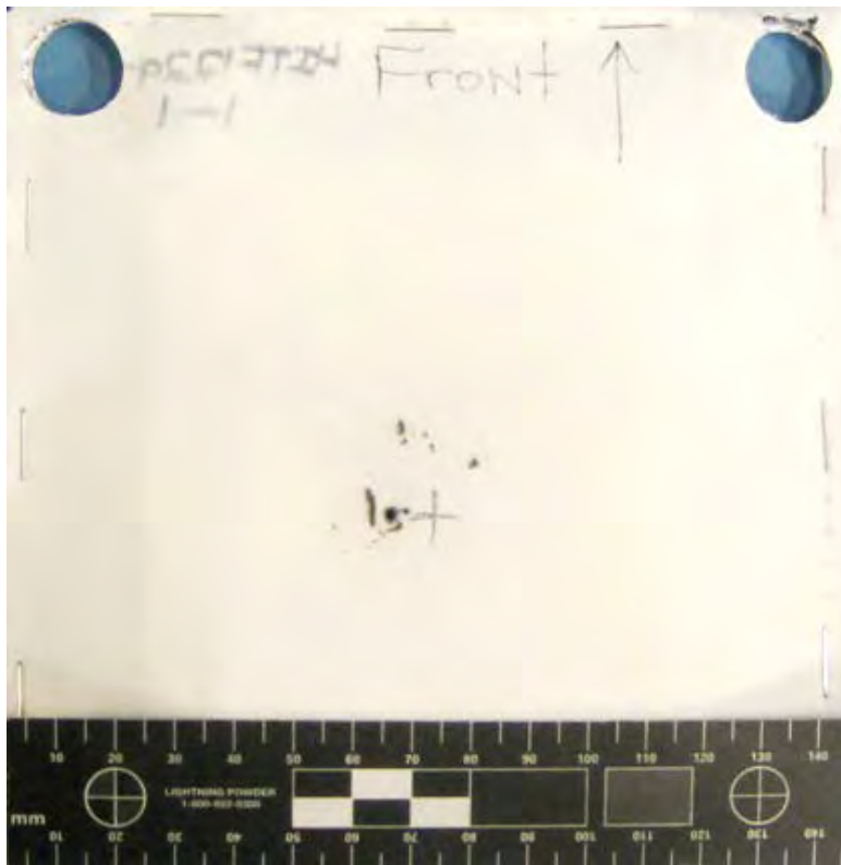
Figure 255 Overall View of Damage to Front of MLI (scale in 5mm increments / black arrow indicates flight path of projectile)
