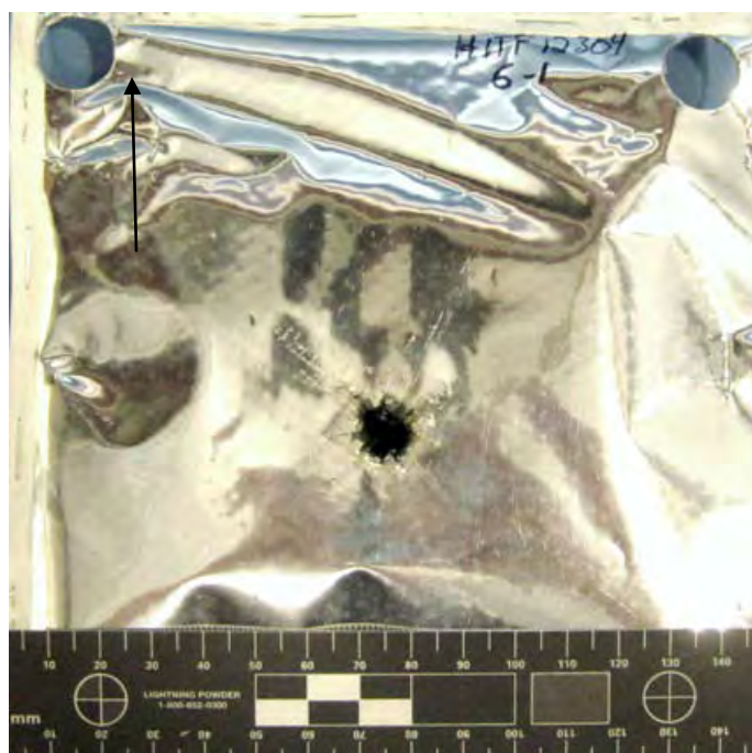
Figure 359 Overall View of Damage to Back Side of MLI (scale in 5mm increments / black arrow indicates flight path of projectile)
