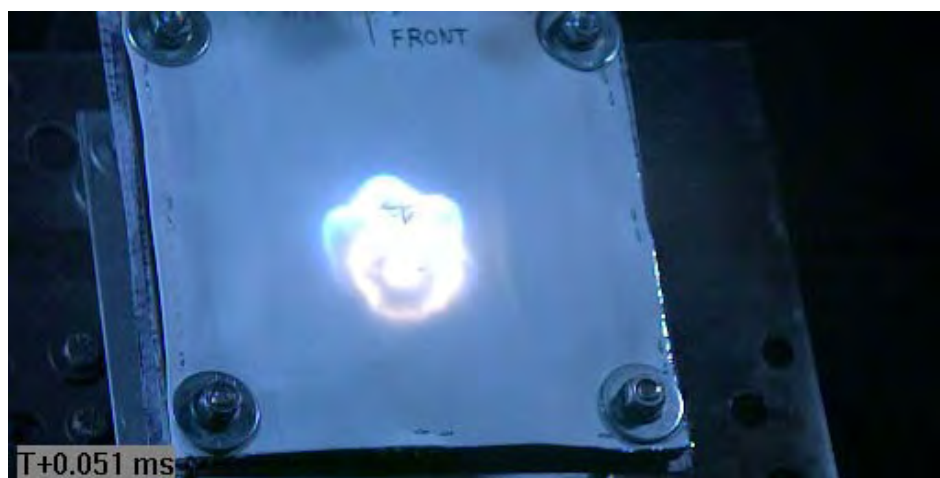
Figure C41 Projectile Impacting Target (via Phantom v711)
