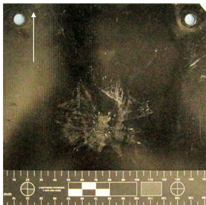
Figure 376 Overall View of Damage to Front of NP 504 Substrate (scale in 5mm increments / white arrow indicates flight path of projectile)
