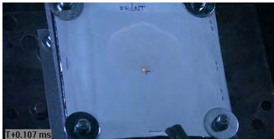
Figure C85 Image of Projectile Impacting Target (via Phantom v711)
