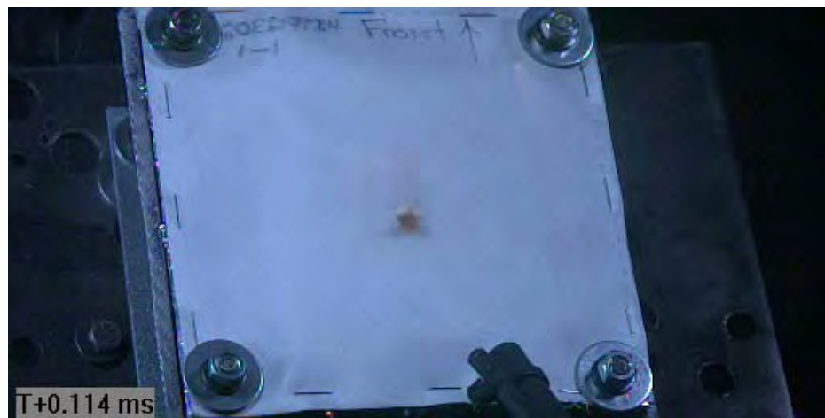
Figure C62 Projectile Impacting Target (via Phantom v711)
