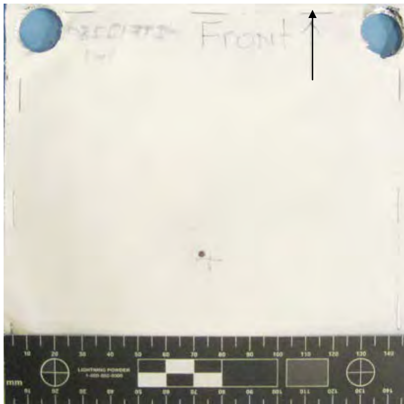
Figure 107 Overall View of Damage to Front of MLI (scale in 5mm increments / black arrow indicates flight path of projectile)
