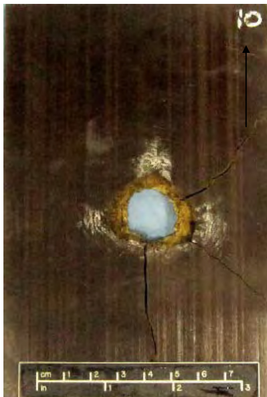
Figure 523 Overall View of Damage to Front of TORLON 5030 Delaminated from Substrate (black arrow indicates flight path of projectile / scale in 1cm increments)
