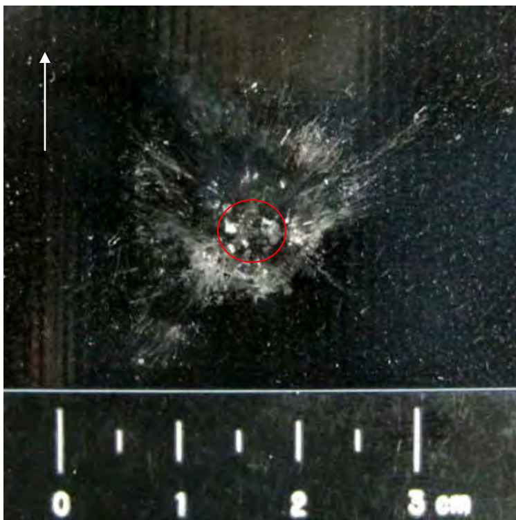
Figure 260 Close-up View of Damage to Front of NP 504 Substrate (scale in 5mm increments / white arrow indicates flight path of projectile)
