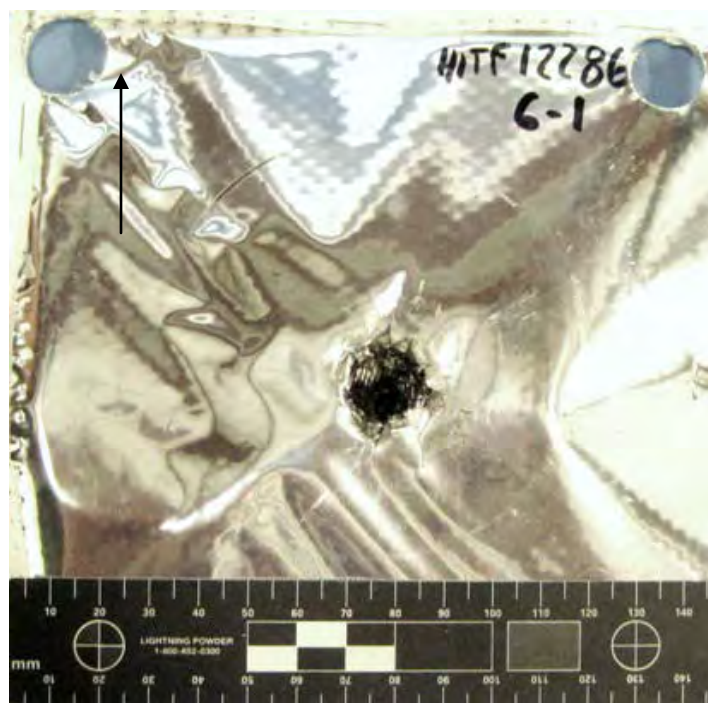
Figure 56 Overall View of Damage to Back Side of MLI (scale in 5mm increments / black arrow indicates flight path of projectile)
