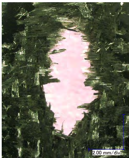
Figure 77 Close-up View of Most Significant Damage to Back Side of NP 504 Substrate (black arrow indicates flight path of projectile / damage within red circle in Figure 76)
