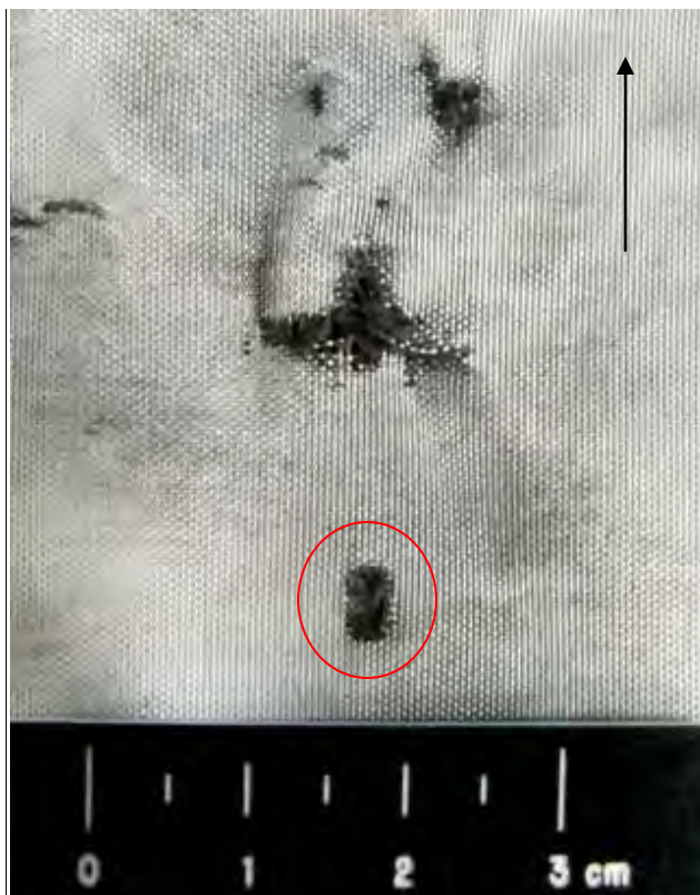
Figure 70 Close-up View of Damage to Front of MLI (scale in 5mm increments / black arrow indicates flight path of projectile / projectile impacted within red circle)
