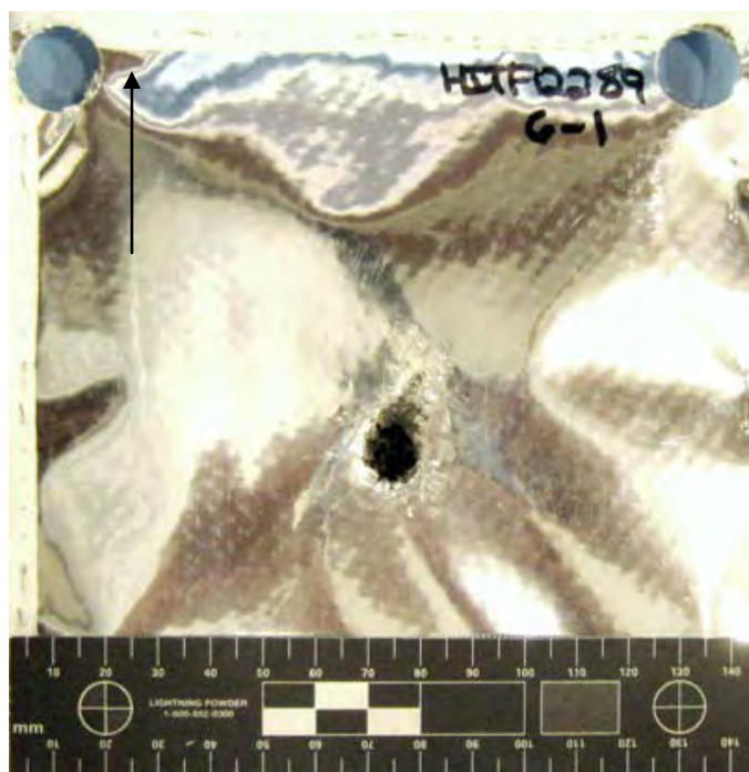
Figure 109 Overall View of Damage to Back Side of MLI (scale in 5mm increments / black arrow indicates flight path of projectile)
