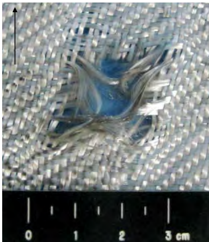
Figure 245 Close-up View of Damage to Back Side of Last Fiberglass Layer (scale in 5mm increments / black arrow indicates flight path of projectile)
