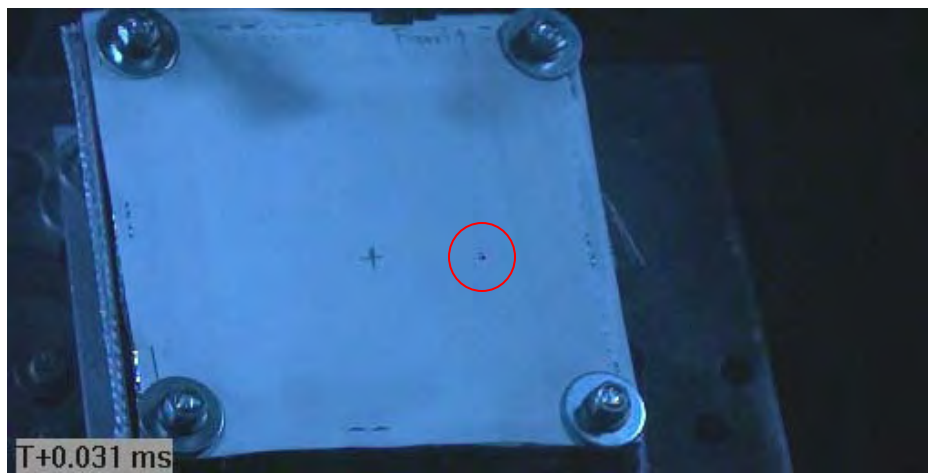
Figure C55 Image of Projectile Captured Prior to Impact (via Phantom v711 / projectile within red circle)
