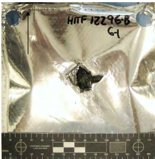
Figure 236 Overall View of Damage to Back Side of MLI (scale in 5mm increments / black arrow indicates flight path of projectile)
