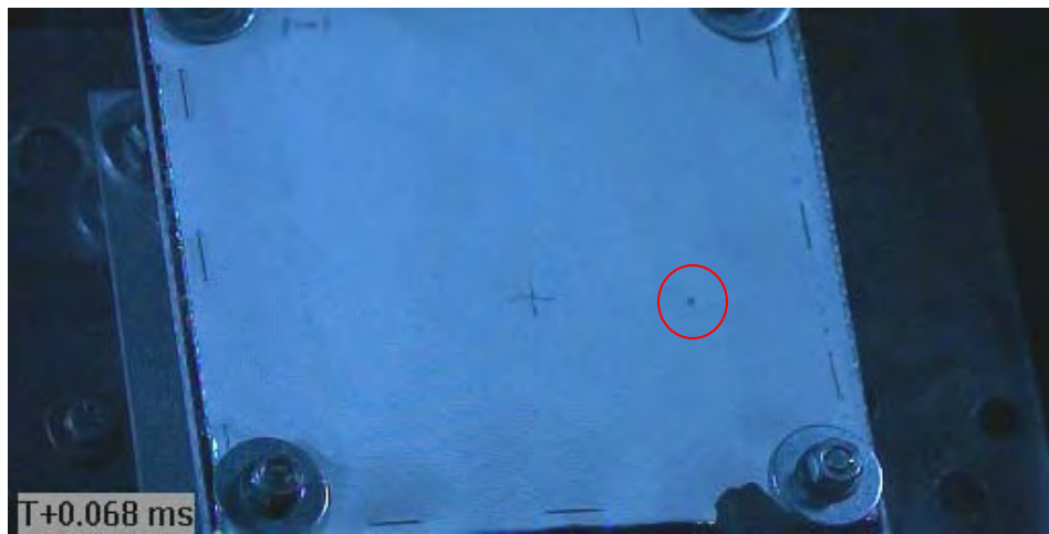
Figure C19 Image of Projectile Captured Prior to Impact (via Phantom v711 / projectile within red circle)
