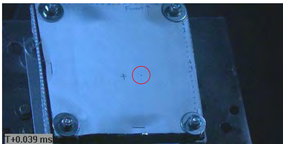
Figure C10 Image of Projectile Captured Prior to Impact (via Phantom v711 / projectile within red circle)
