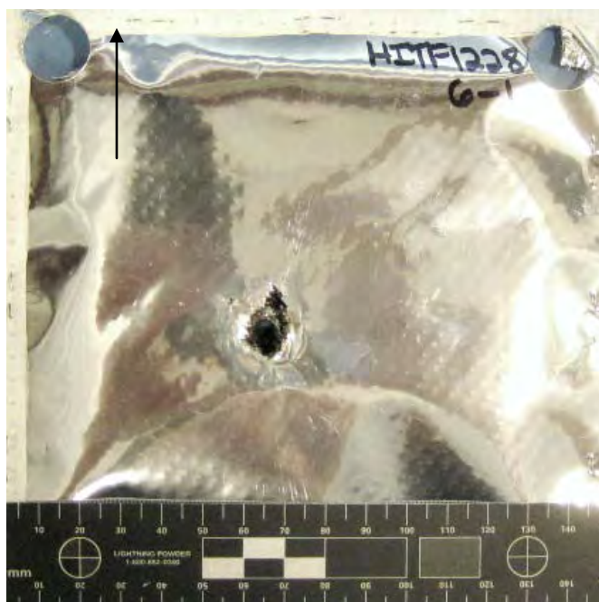
Figure 26 Overall View of Damage to Back Side of MLI (scale in 5mm increments / black arrow indicates flight path of projectile)
