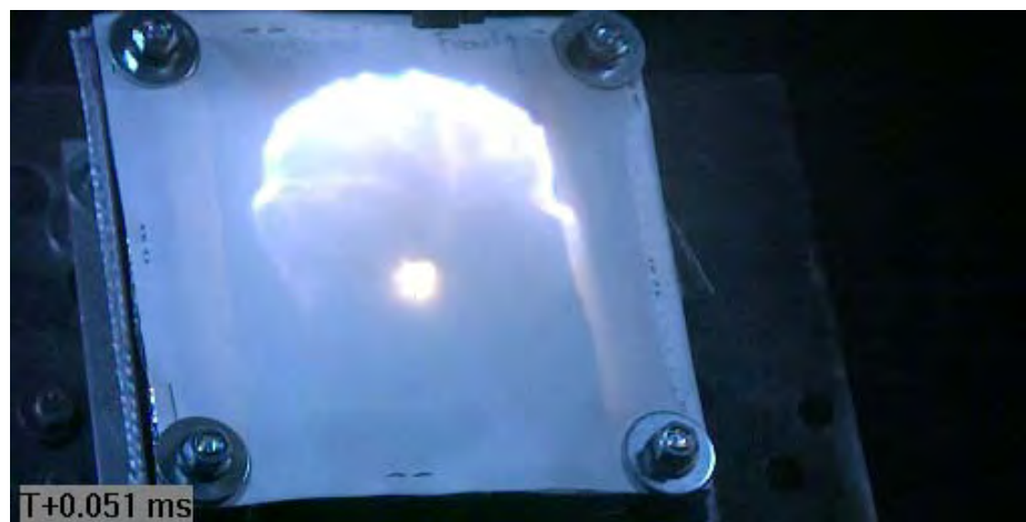
Figure C56 Projectile Impacting Target (via Phantom v711)
