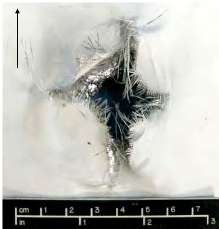
Figure 547 Close-up View of Damage to Front of MLI (scale in 5mm increments / black arrow indicates flight path of projectile)
