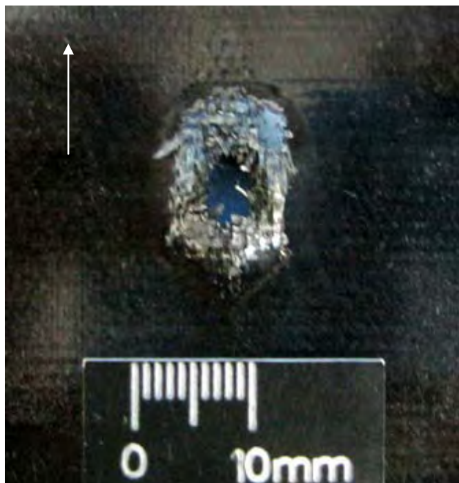
Figure 328 Close-up View of Damage to Back Side of NP 504 Substrate (scale in 1mm increments / white arrow indicates flight path of projectile)
