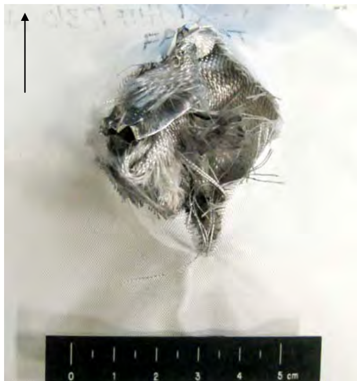
Figure 471 Close-up View of Damage to Front of MLI (scale in 5mm increments / black arrow indicates flight path of projectile)
