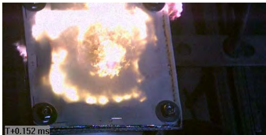
Figure C73 Projectile Impacting Target (via Phantom v711)
