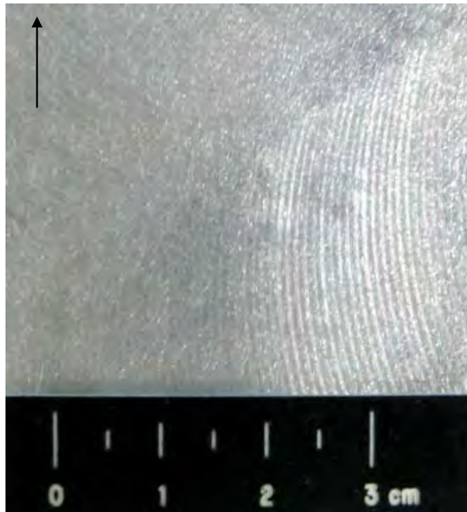
Figure 405 Close-up View of Damage on Back Side of Rear Wall (scale in 5mm increments / black arrow indicates flight path of projectile)
