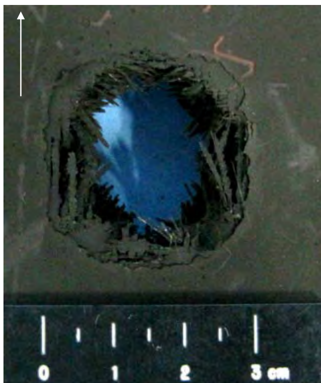
Figure 528 Close-up View of Damage to Front NP 504 Substrate with TORLON 5030 Delaminated (scale in 5mm increments / white arrow indicates flight path of projectile)
