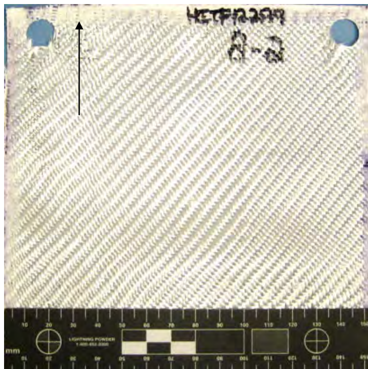
Figure 289 Overall View of Damage to Back Side of 2 nd Fiberglass Layer (scale in 5mm increments / black arrow indicates flight path of projectile)
