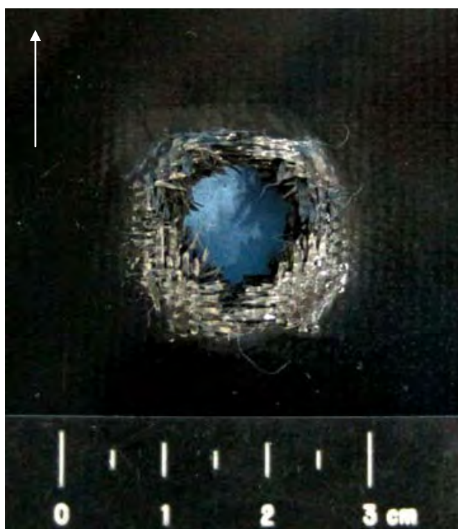
Figure 395 Close-up View of Damage to Back Side of NP 504 Substrate (scale in 1mm increments / white arrow indicates flight path of projectile)
