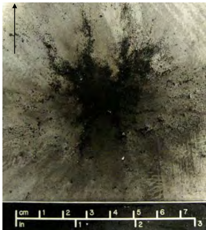
Figure 400 Close-up View of Damage to Front of Rear Wall (scale in 1cm increments / black arrow indicates flight path of projectile / uncleaned)
