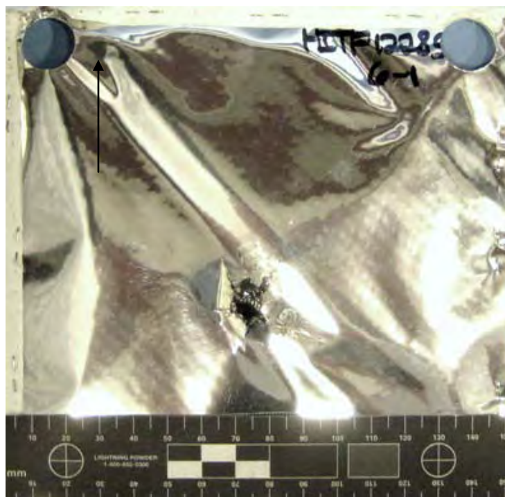
Figure 41 Overall View of Damage to Back Side of MLI (scale in 5mm increments / black arrow indicates flight path of projectile)
