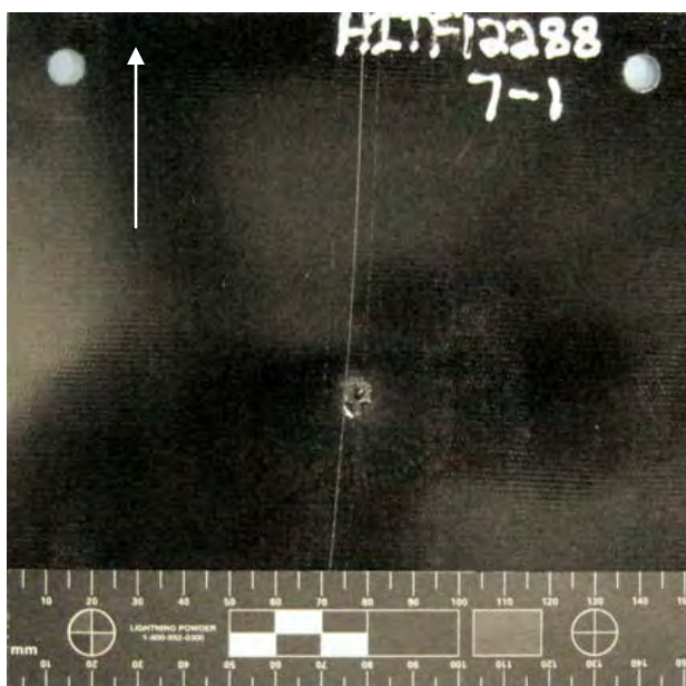
Figure 94 Overall View of Damage to Back Side of NP 504 Substrate (scale in 5mm increments / white arrow indicates flight path of projectile)
