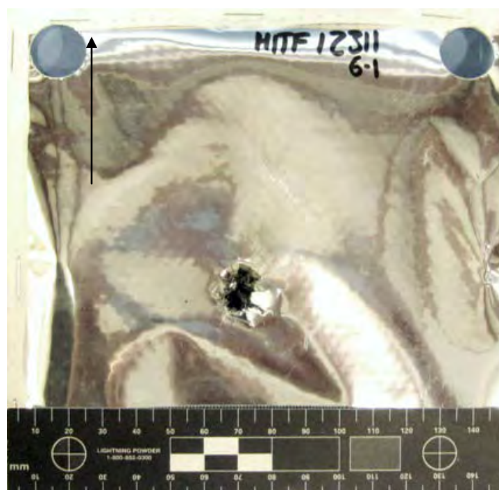
Figure 491 Overall View of Damage to Back Side of MLI (scale in 5mm increments / black arrow indicates flight path of projectile)
