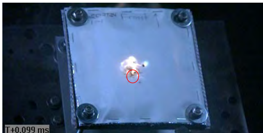
Figure C47 Image of Projectile and Secondary Debris Impacting Target (via Phantom v711 / projectile impacting within red circle, the remaining impacts are secondary debris)
