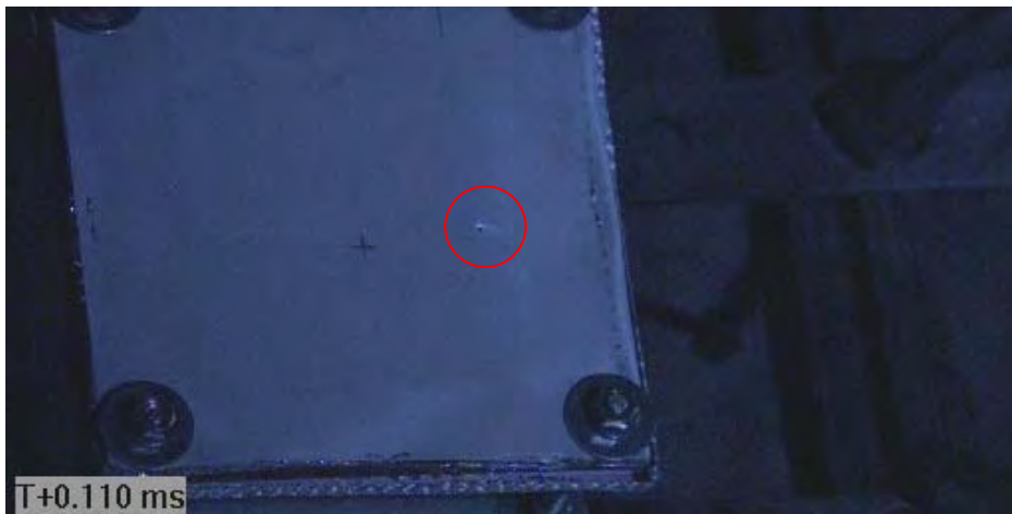
Figure C31 Image of Projectile Captured Prior to Impact (via Phantom v711 / projectile within red circle)
