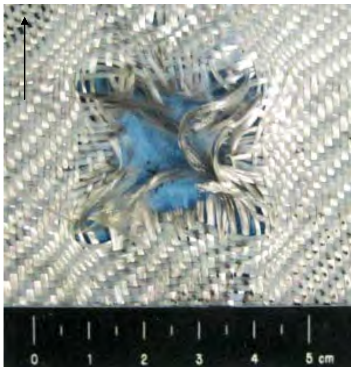
Figure 398 Close-up View of Damage to Back Side of Last Fiberglass Layer (scale in 5mm increments / black arrow indicates flight path of projectile)
