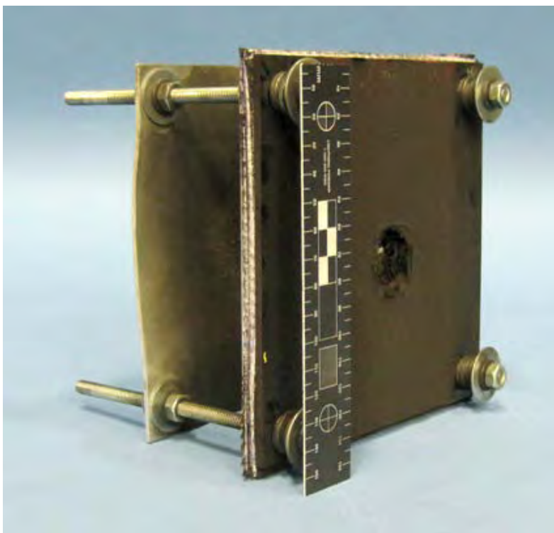
Figure 521 Overall Oblique Front View of Sample (scale in 5mm increments / with TORLON 5030 and MLI displaced from test configuration)
