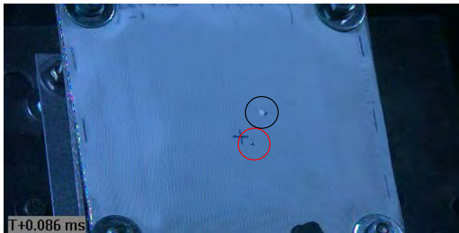
Figure C16 Image of Projectile and Sabot Petal Captured Prior to Impact (via Phantom v711 / projectile within red circle / sabot petal within black circle)
