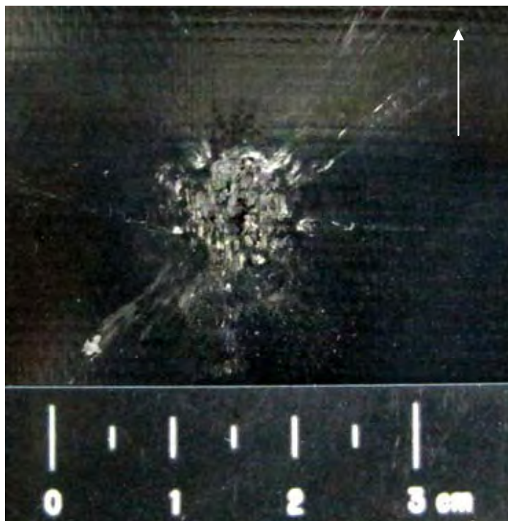
Figure 362 Close-up View of Damage to Front of NP 504 Substrate (scale in 5mm increments / white arrow indicates flight path of projectile)
