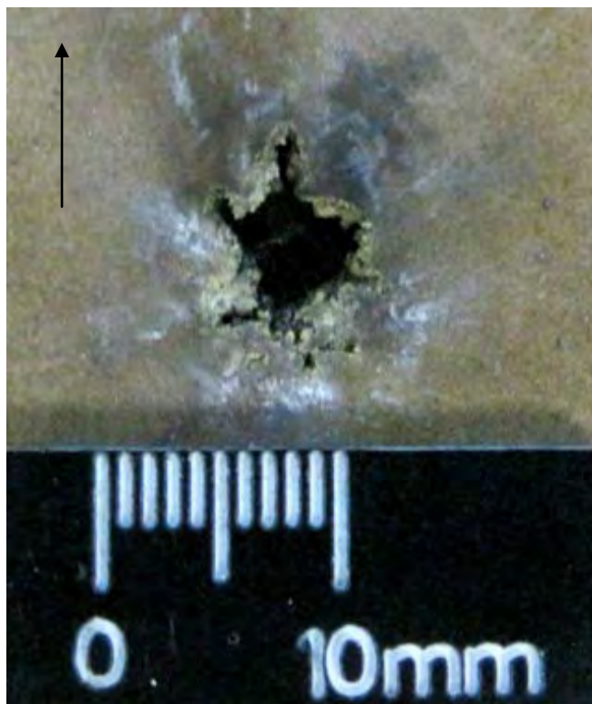
Figure 299 Close-up View of Damage to Front of TORLON 5030 (scale in 5mm increments / white arrow indicates flight path of projectile)
