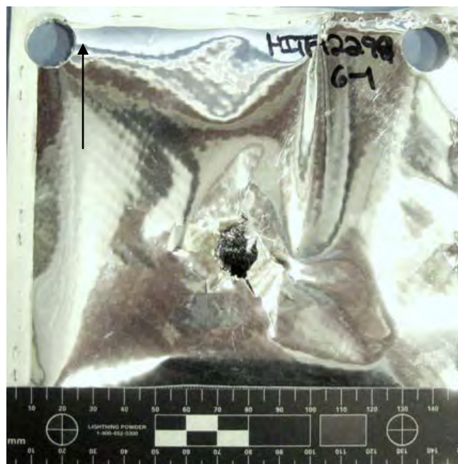
Figure 281 Overall View of Damage to Back Side of MLI (scale in 5mm increments / black arrow indicates flight path of projectile)
