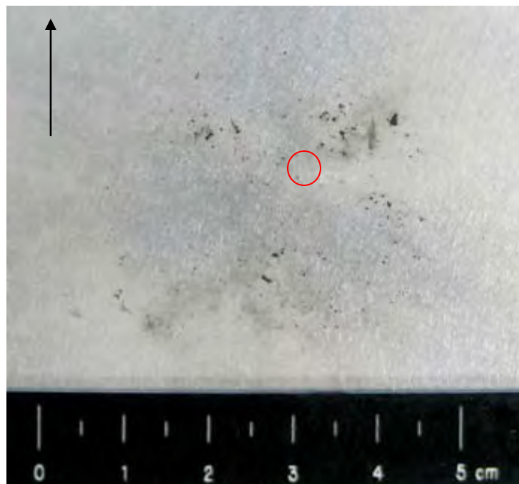
Figure 351 Close-up View of Damage to Front of Rear Wall (scale in 5mm increments / black arrow indicates flight path of projectile)
