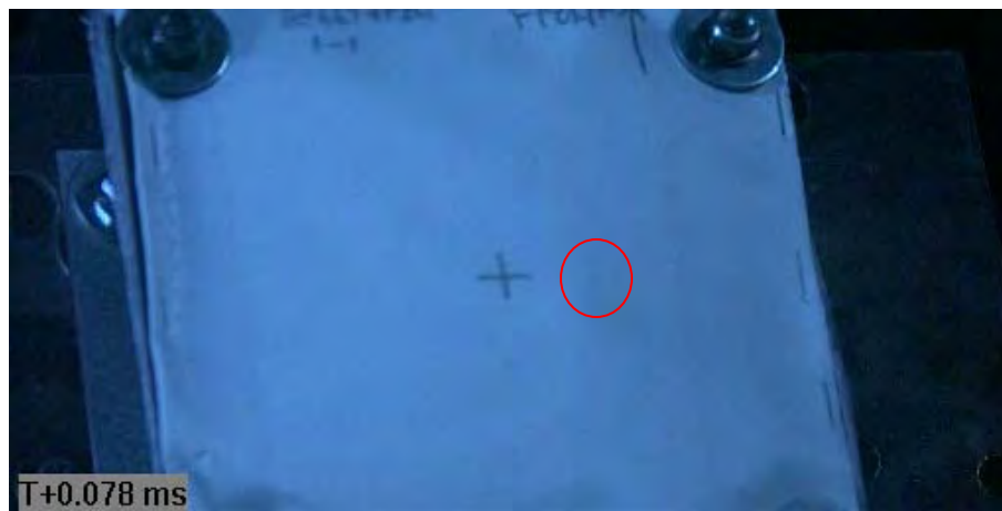
Figure C2 Faint Image of Projectile Captured Prior to Impact (via Phantom v711 / projectile within red circle)
