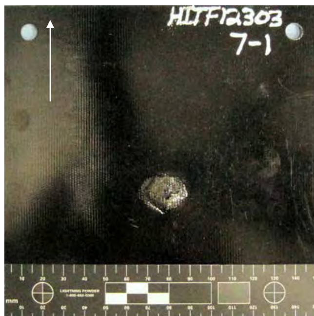
Figure 345 Overall View of Damage to Back Side of NP 504 Substrate (scale in 5mm increments / white arrow indicates flight path of projectile)
