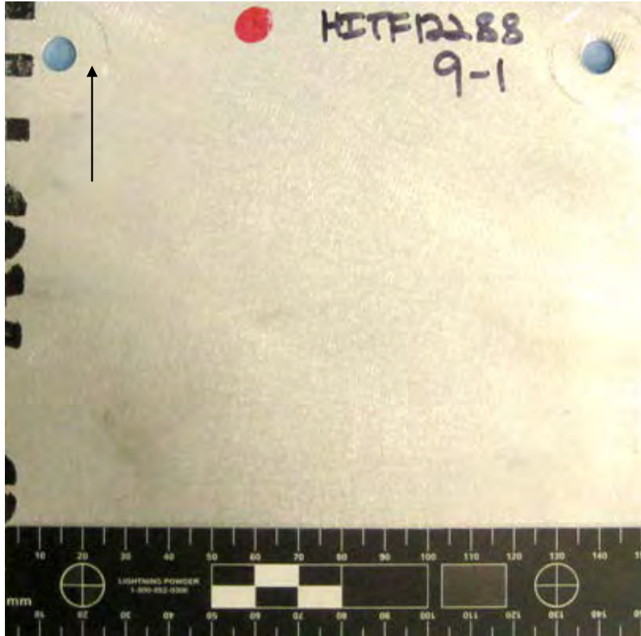
Figure 103 Overall View of Damage to Front of Rear Wall (scale in 5mm increments / black arrow indicates flight path of projectile)
