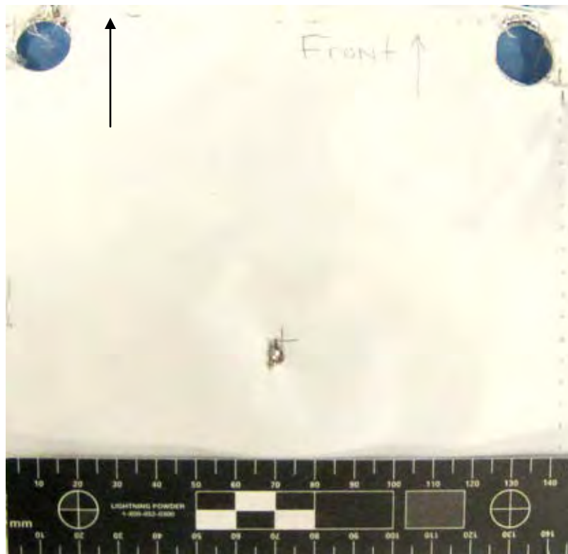
Figure 410 Overall View of Damage to Front of MLI (black arrow indicates flight path of projectile / scale in 5mm increments)
