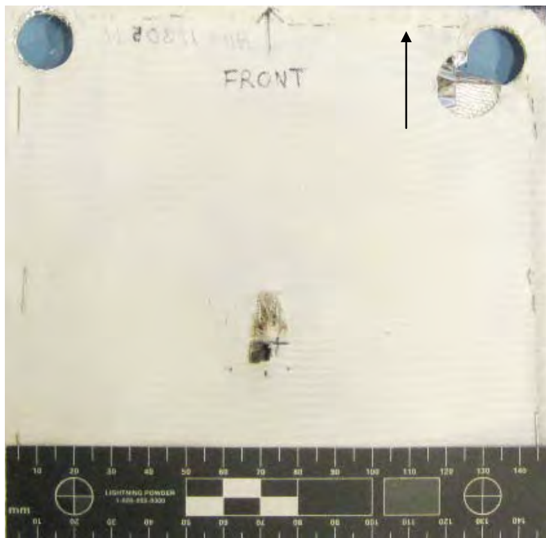
Figure 372 Overall View of Damage to Front of MLI (scale in 5mm increments / black arrow indicates flight path of projectile)
