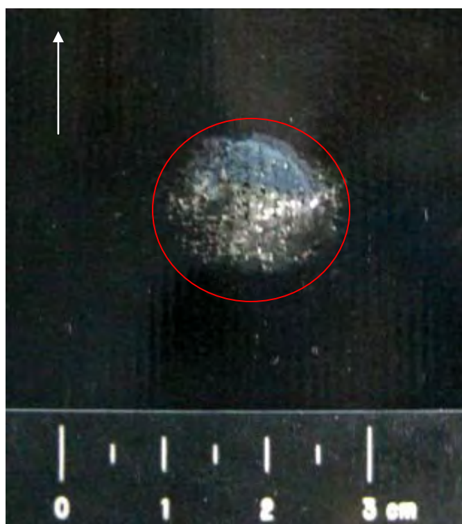
Figure 514 Close-up View of Damage to Back Side of NP 504 Substrate (scale in 5mm increments / white arrow indicates flight path of projectile)
