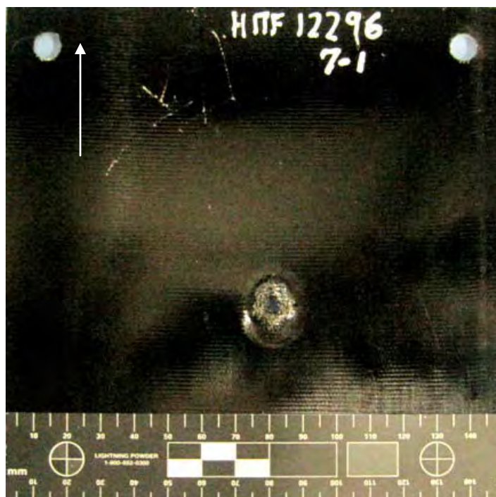
Figure 221 Overall View of Damage to Back Side of NP 504 Substrate (scale in 5mm increments / white arrow indicates flight path of projectile)
