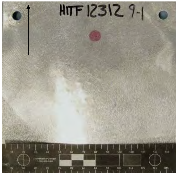
Figure 539 Overall View of Damage to Back Side of Rear Wall (scale in 5mm increments / black arrow indicates flight path of projectile)
