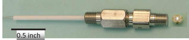
Figure 6: Spark-plug type package for high temperature SiC capacitive pressure sensor [11].
