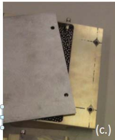
Figure 8. Bracket Type Particle Damper Assembly (a.) Installed Bracket. (b.) Bathtub Cavity in Bracket. (c.)Bracket with Cover. (d.) Bracket filled with BB type Particles.
