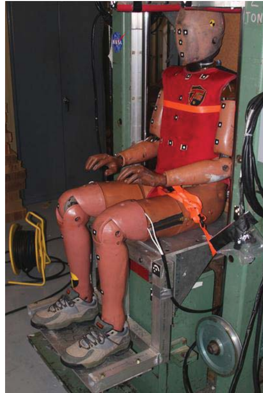
Figure 21- THOR test setup with footrest
