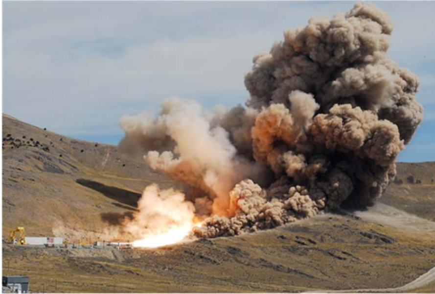
Figure 1. Typical Motor Firing into Hill Behind T-97 Showing Motor Exhaust and Particulates Shortly After Start
