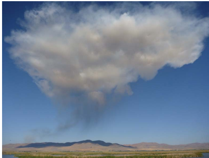
Figure 2. Precipitating Cloud and Debris Trail Produced by a Five-Segment Motor Tested at T-97
