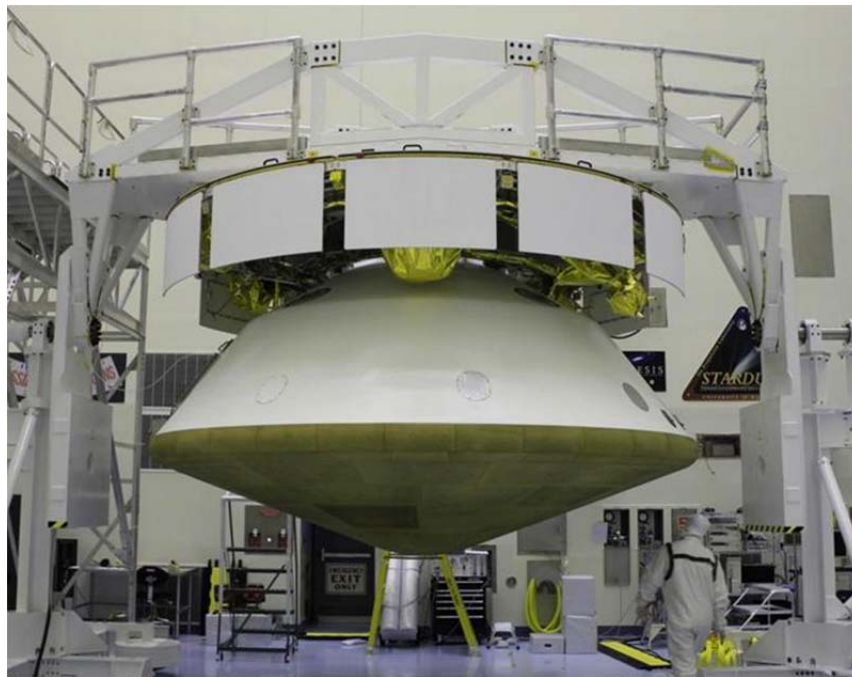
Figure 3. Cruise configuration in testing. Image credit: NASA/JPL-Caltech
