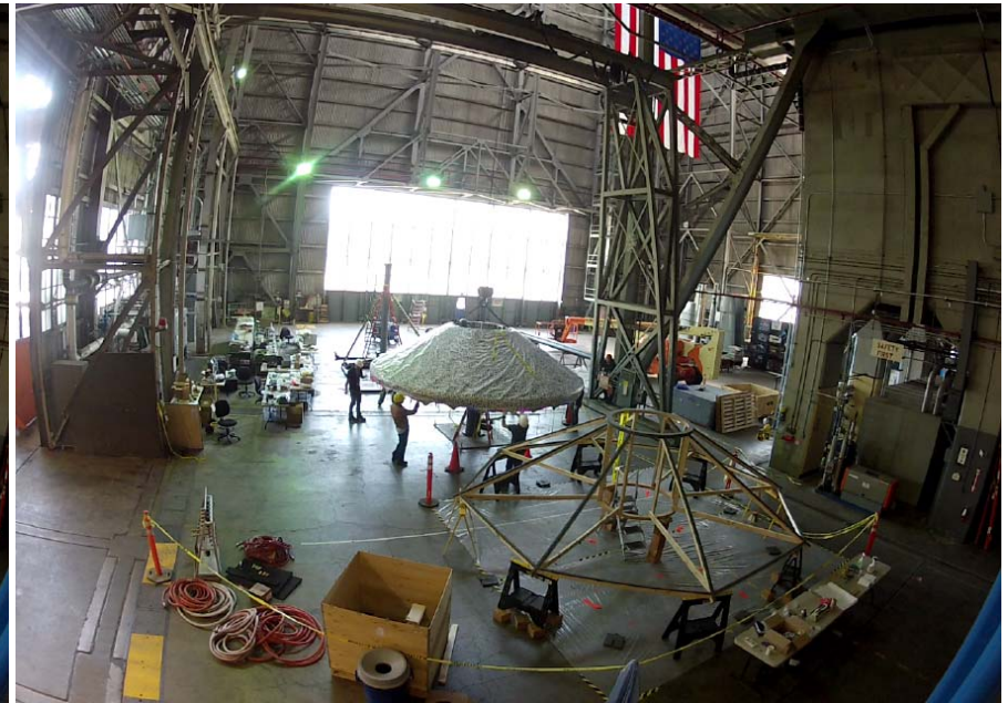
Aerocover Secured to 6 m Test Article
