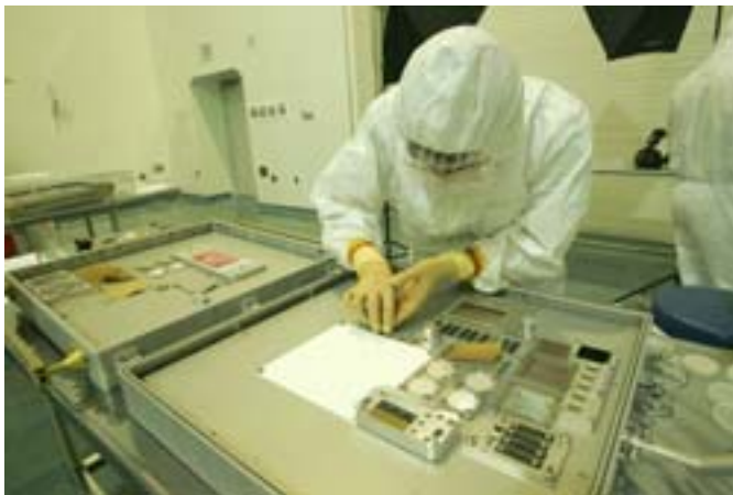
Miria Finckenor, materials engineer at the Marshall Space Flight Center, removes a sample from a Materials International Space Station Experiment (MISSE) Passive Experiment Container at Langley Research Center. Approximately 35 members of the MISSE team traveled from across the country to witness the "grand opening" of MISSE-1 and 2 in 2005. (NASA/Jeff Caplan)
