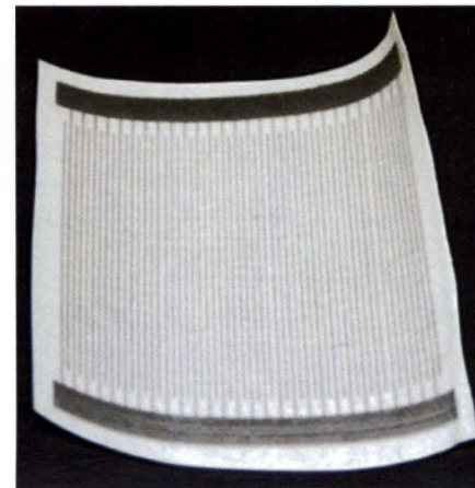
Two EDS panels for thermal radiators
