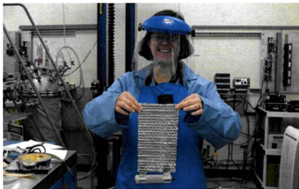
Figure 5a: Here, I am testing the tape. The tape is attached to the Mylar and is pulled down by a weight
