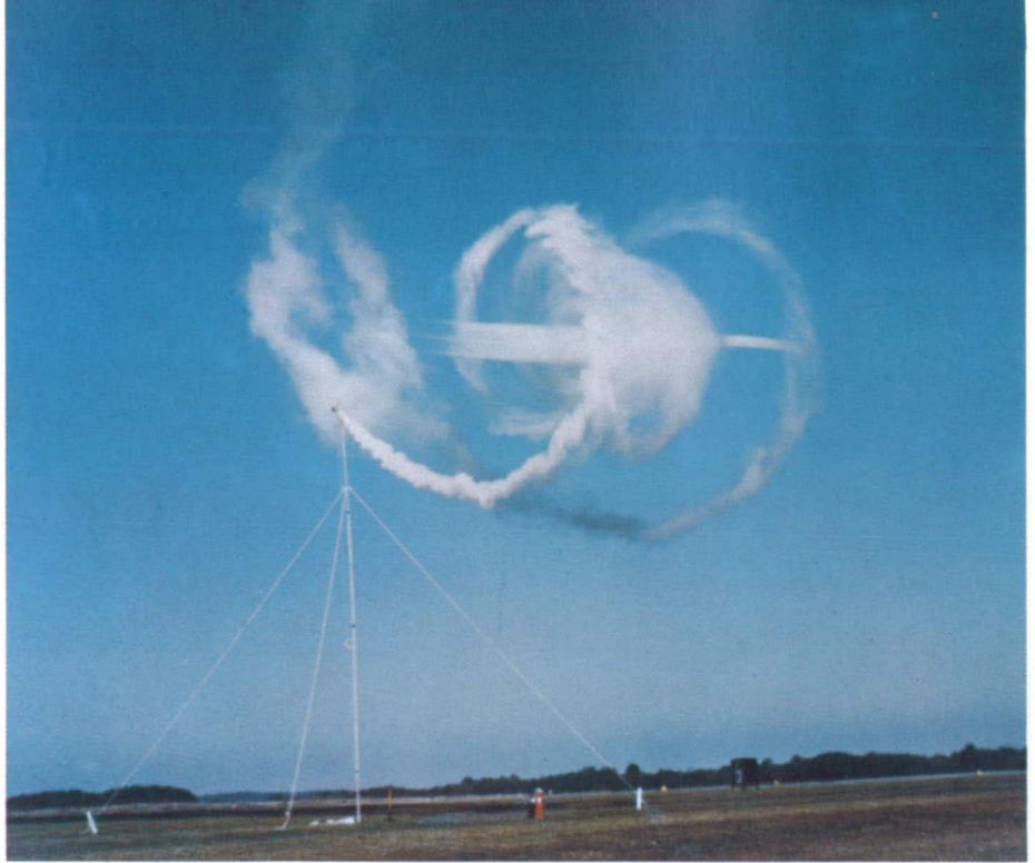
In this test, the trailing vortex is made visible by smoke injection, providing an indication of the scope of this "horizontal whirlwind."
