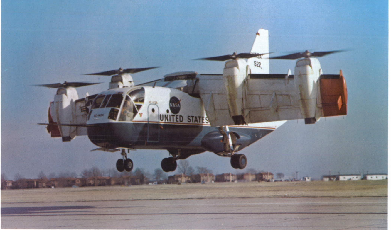
The XC-142A tilt-wing vertical/short takeoff and landing (V/STOL) aircraft taking off for a test flight at Langley Research Center.
