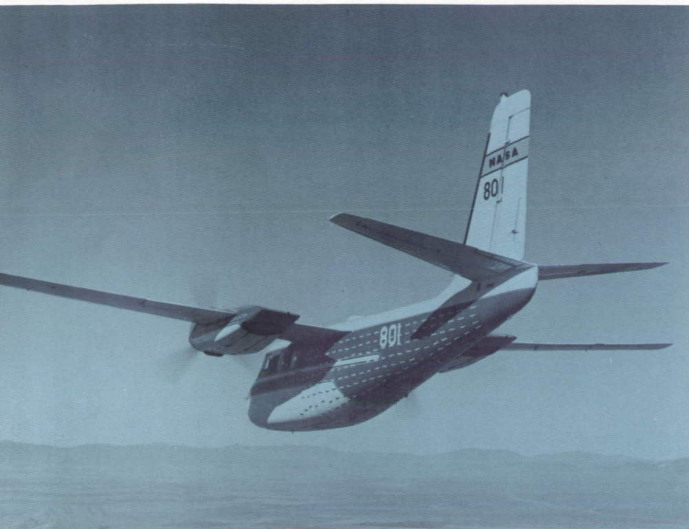
Light twin-engine general aviation aircraft are evaluated in flight at the Flight Research Center in a program aimed at improving operational efficiency. In the test flight illustrated here tufts of fiber have been affixed along the sides of the fuselage to provide measurements of air flow across the surface.
