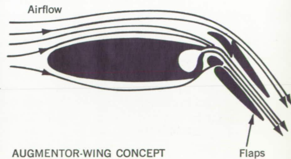
The augmentor wing concept was tested in model form in the full scale tunnel at Ames Research Center.
