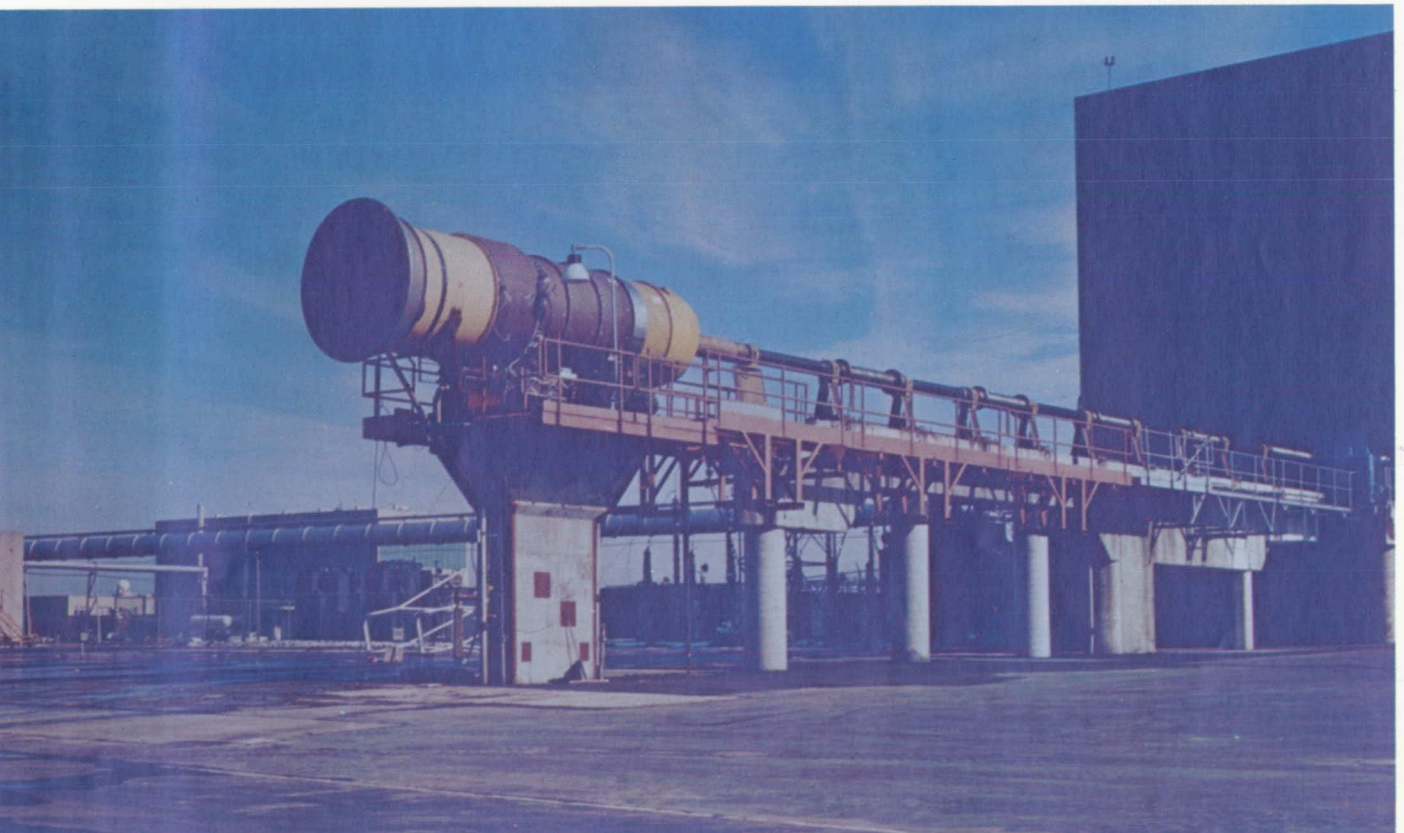
Fan test stand at Lewis Research Center is used in developmental testing of fan configurations in the noise-reaction program.
