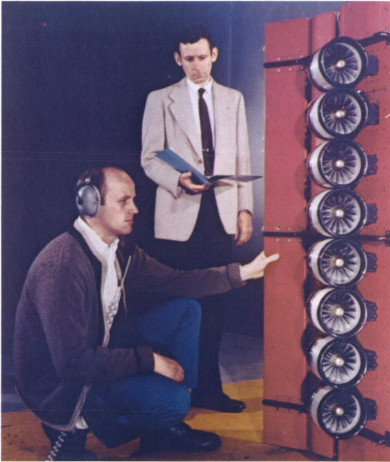
Generalized model of an externally blown flap is studied in a Lewis Research Center wind tunnel.
