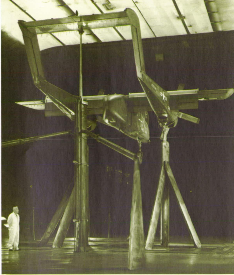
A rotating-cylinder flap concept was tested in an Ames Research Center wind tunnel both in small scale and in full scale as shown here.
