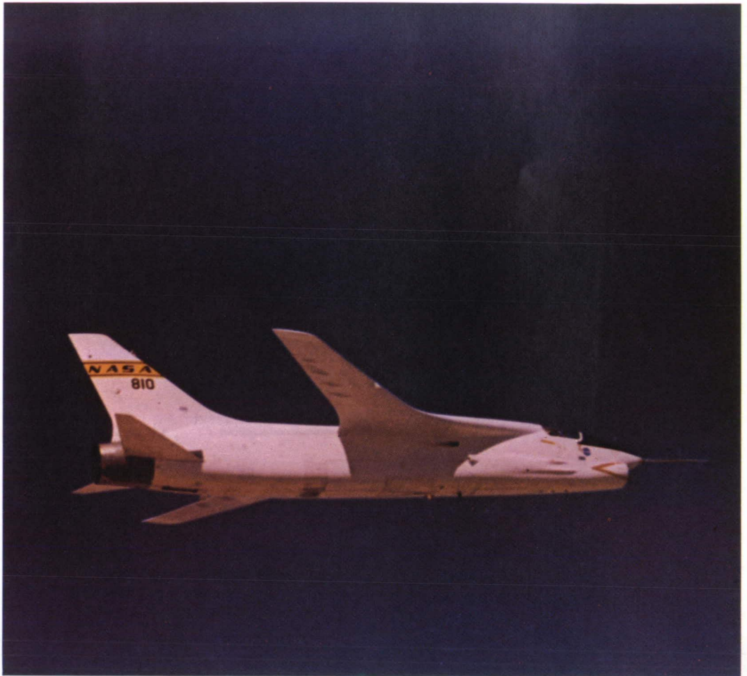
The NASA supercritical wing is being flight tested by NASA's Flight Research Center aboard an extensively modified TF-8A jet trainer.
