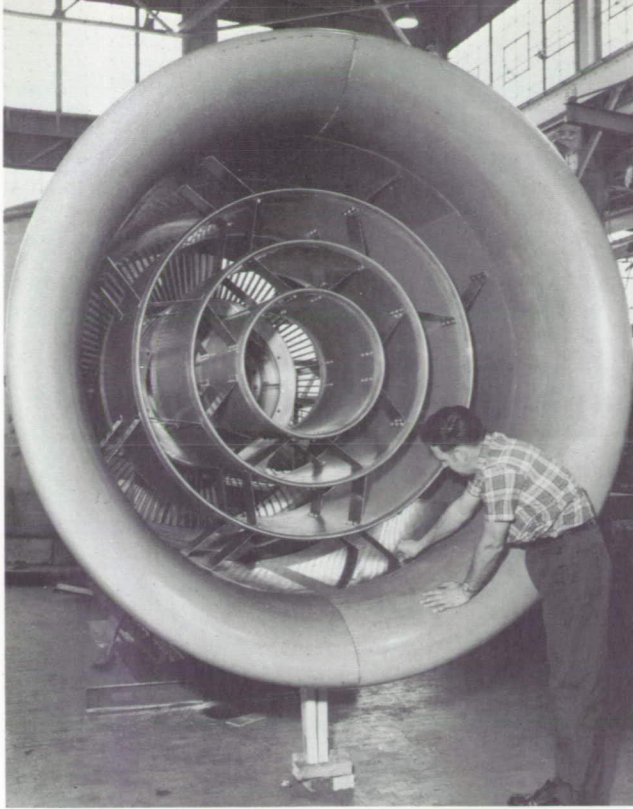
Acoustically damped development inlet configuration shows one current approach to reducing jet engine noise.
