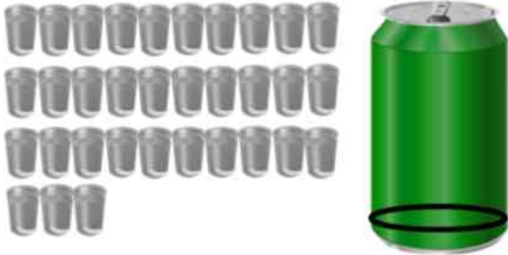
Figure 20-2: Following the propellant anomaly, the attitude control system (ACS) algorithms were adjusted to be miserly with the remaining propellant. I had calculated that we got LCROSS’s usage down to ~33 thimbles of fuel a day (40grams/day of hydrazine) or the equivalent of a tenth of a can of soda:
