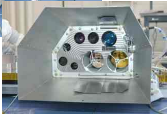
Figure 10-4: LCROSS Payload Observation Deck, “POD.”
