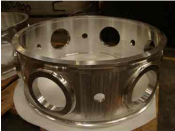
Figure 10-5: LCROSS ESPA ring freshly machined.
