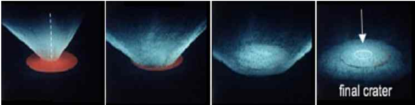
Figure 21-7: NASA-ARC Ames Vertical Gun Range (AVGR) facility impact testing (Images courtesy of Peter Shultz).
