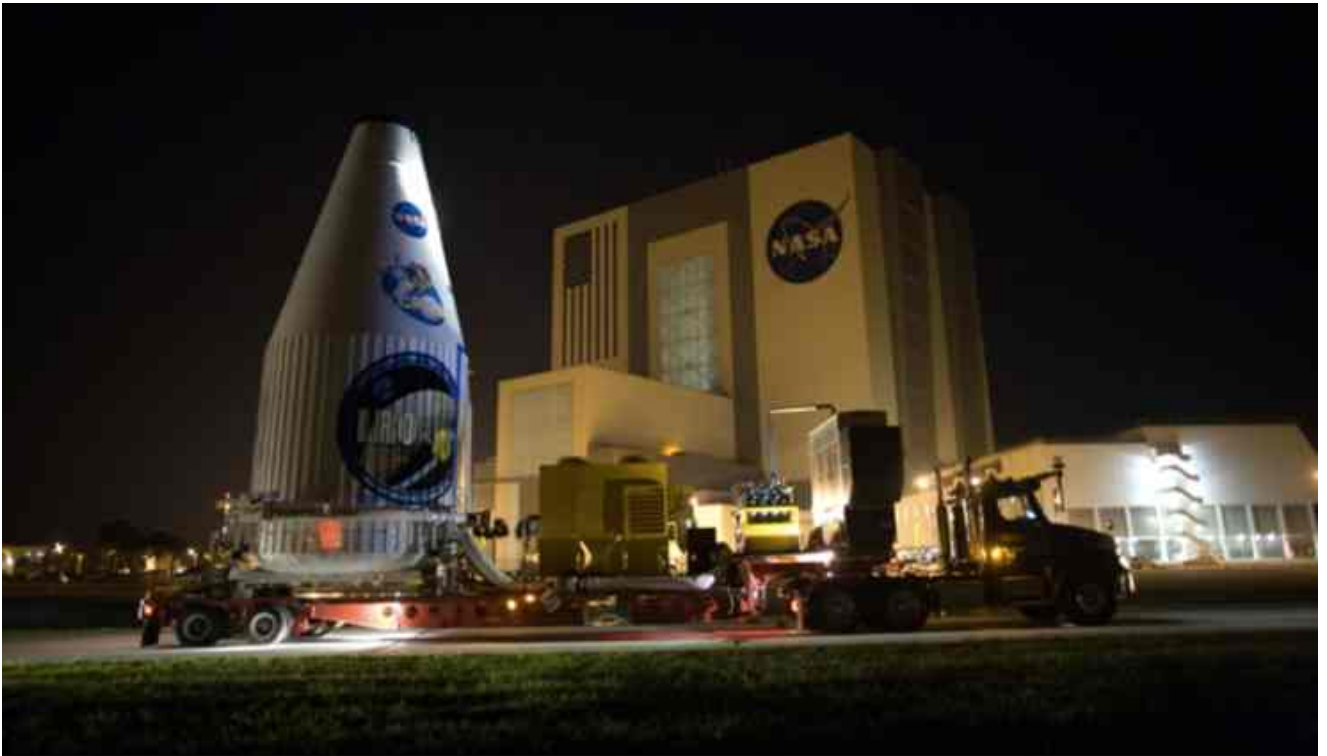
Figure 16-1: LCROSS/LRO packed in the launch fairing, moving out to the launch pad for integration with the launch vehicle.
