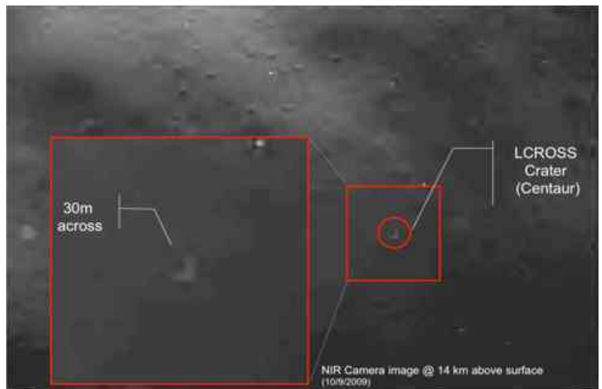
Figure 18-9: NIR Camera image of LCROSS Centaur Impact crater @ 14 km above surface, 2009-10-09.
