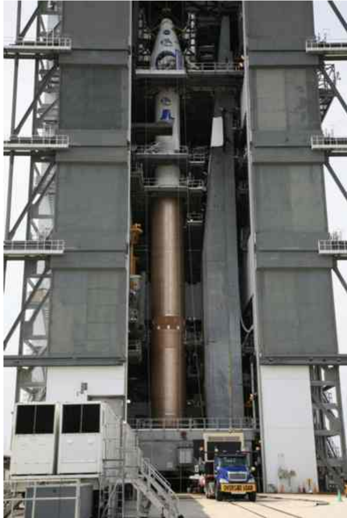
Figure 16-2: LCROSS/LRO stacked atop the Atlas-V launch vehicle at the Vertical Integration Facility (VIF), Space Launch Complex 41, Cape Canaveral.
