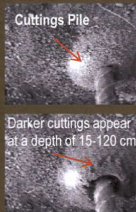
Auger and Examine Cutting Pile for Ice with Near Infrared Spectrometer
