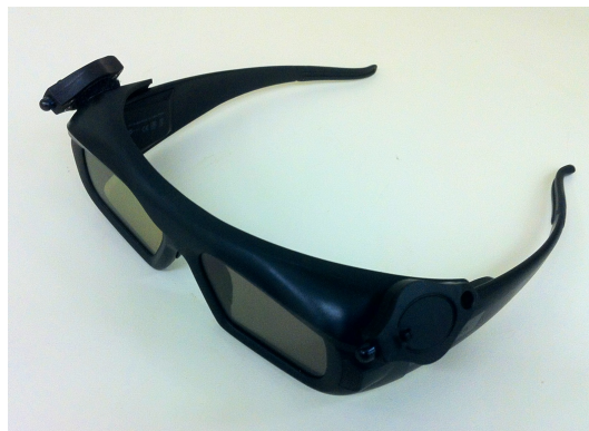
Figure 1. Modified stereo glasses with velcro-fastened switched LED keychains with 950nm infrared bulbs. Each keychain is powered by two 3V lithium CMOS batteries.
