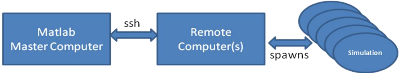
Figure 3. High level view of end to end code architecture. The central manager spawns parallel simulations on remote hosts.
