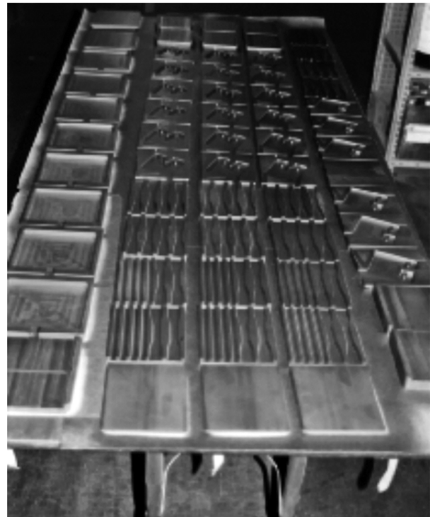
Figure 2.—Graphite mold cavities used to cast test specimens.
