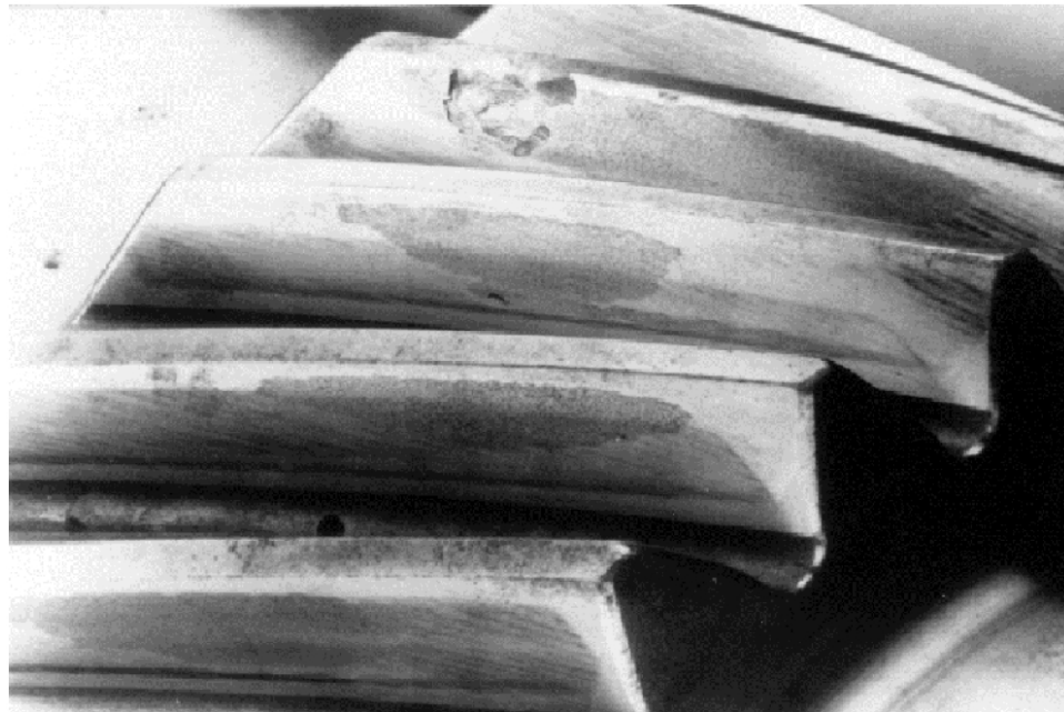
Figure 9.—Example of Micropitting. Extracted from ANSI/AGMA 1010-E95, Appearance of Gear Teeth Terminology of Wear and Failure, with the permission of the publisher, the American Gear Manufacturers Association, 1500 King Street, Suite 201, Alexandria, Virginia 22314.
