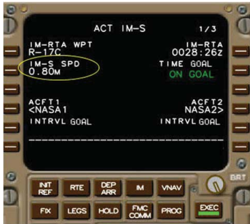
Figure 7. FIM Commanded End Speed shown on MCDU.
