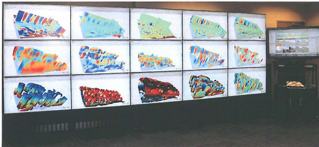
Figure 5. The DV3D distributed visualization framework deployed on the NASA NCCS hyperwall. This configuration enables scientists to exploit the full capacity of the NCCS hyperwall cluster (32 dual-core Xeon Harpertown processors, 16 Quadro FX 1700 GPUs, and a 17 by 6-foot, 15.7 million pixel display) in support of interactive visual data analysis and understanding of very complex climate datasets.
