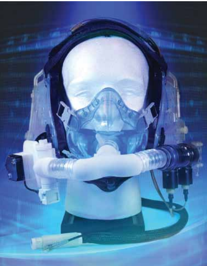
NASA's Portable Unit for Metabolic Analysis (PUMA) uses miniaturized sensors to measure a person's metabolic rate.
