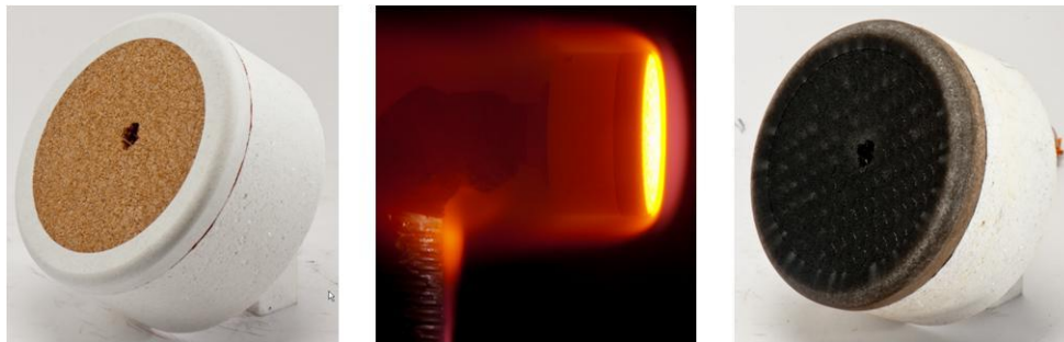
Figure 21: SLA sample before, during, and after the arcjet test.
