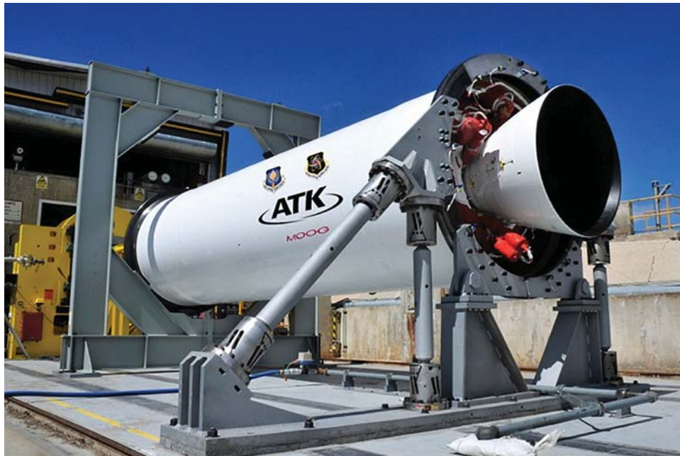
Figure 50. ATK ABEDRR LSC-1 92-in-diameter test motor.
