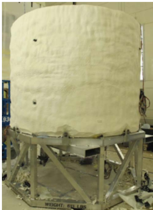
Figure 10. Foam insulated cryotank test article.
