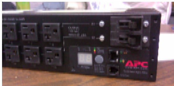
Figure 3.—APC AP7902 power distribution unit (PDU).
