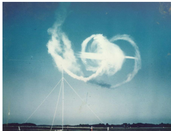
Figure 1. Wake vortex experiment conducted at NASA Langley Research Center in the early 1970s. Axial flows can be seen at the center of the vortex.
