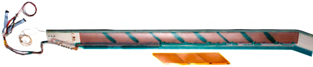
Figure 2. ATR blade shown with piezoelectric actuators.
