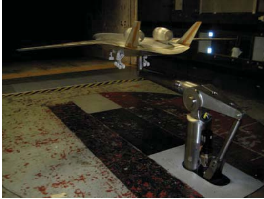
Figure 16. The 5.8% HWB model mounted on the aerodynamic support system installed on model cart #1 in the 14x22 Tunnel. Photograph by George Holmich.
