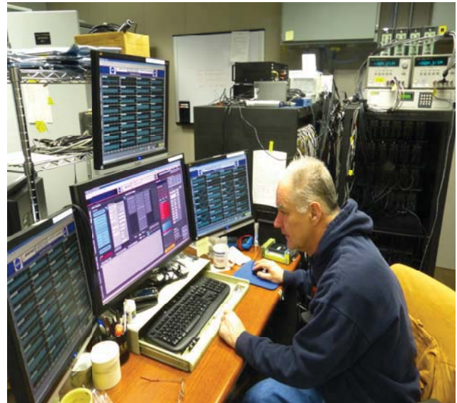
Figure 21. Data acquisition system main data control computer for the HWB Test. Four monitors are used to track acquired data streams during testing.
