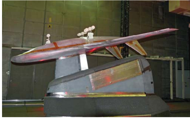
Figure 17. Acoustic model support with fairing and acoustic treatment applied. Photograph by George Holmich.
