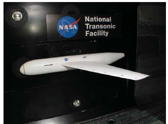
Figure 6: FAST-MAC model in cruise configuration mounted on the sidewall in the NTF.
