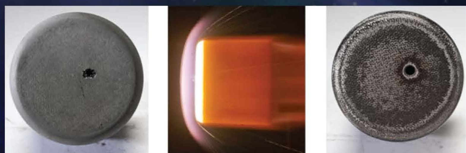
Carbon-Carbon test sample, before, during, and after arc-jet testing.
