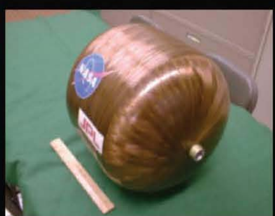
5-mil Aluminum liner, PBO composite
