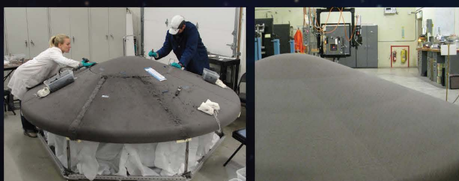
High performance aeroshell assembly (seem packing)
