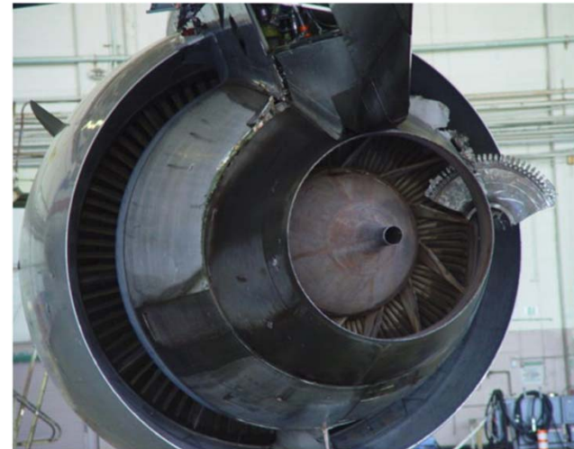
Turbine Disk Failure – June 2, 2006
