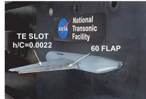
Figure 8. FAST-MAC model mounted in the NTF test section.
