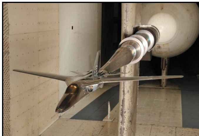
Figure 2. F-111 test article. Wing sweep of 35^{\circ} , 48-inch wing span
