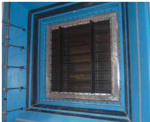
Figure 5: Vertical array of five intensity probes (left side) used for TL testing. A PRSEUS composite test panel is shown installed in the aluminum/MDF sandwich adapter frame.
