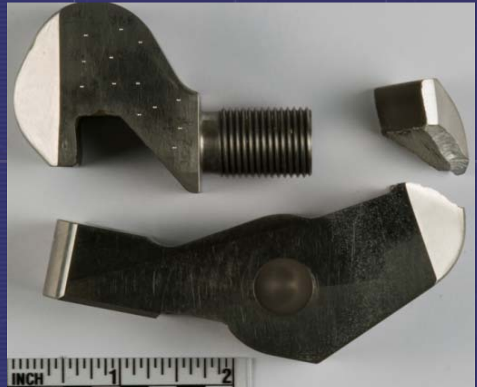
Active latch hook static load failure location at the hook ledge transition radius.
