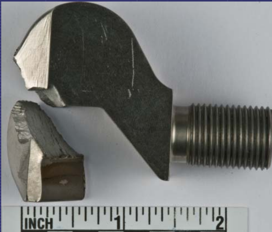
Passive latch hook static load failure location at the hook ledge transition radius.
