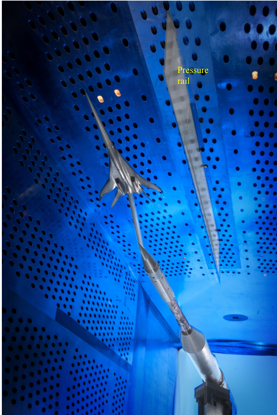
Figure 2.—Boeing N+2 validation model and 14-in. sonic boom pressure rail installed in the 8x6 SWT.
