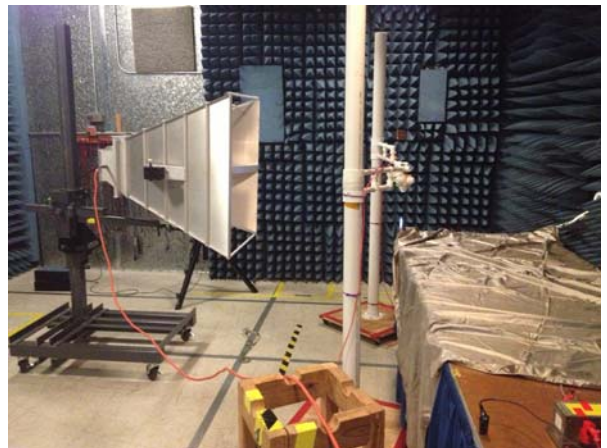
Figure 4: Above, is showing the instrumentation used to perform the EMI tests.
