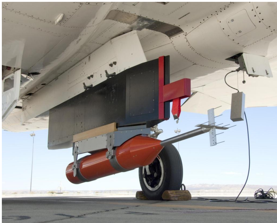
Figure 2. The experiment setup for local flow investigation prior to inlet flight-testing.
