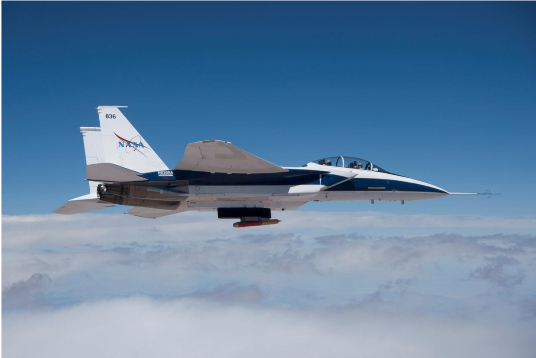
Figure 1. The NASA F-15B, tail number 836, during the first channeled center-body inlet investigation flight.
