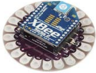
Xbee radio mounted on a LilyPad Xbee breakout board
