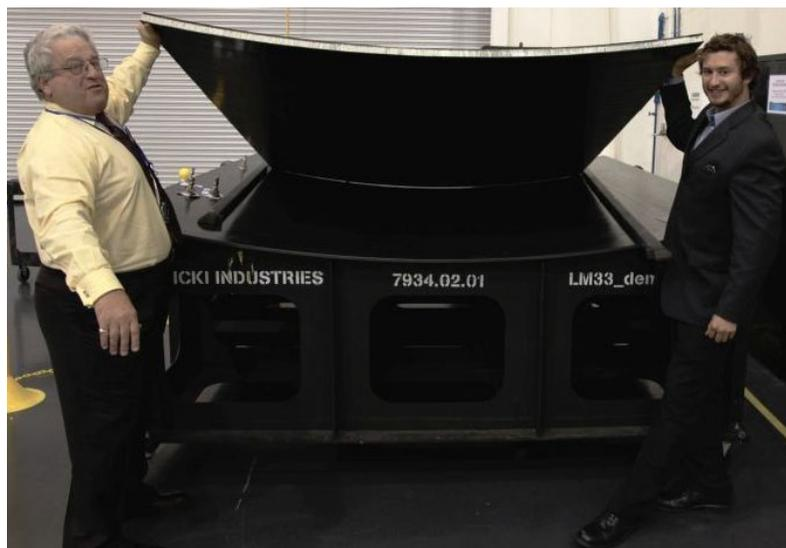
Figure 1.—Cured 1/16<sup>th</sup> arc segment panel and the tool it was molded on.
