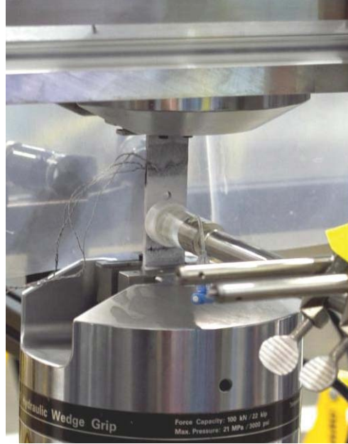
Fig. 17. Non-immersion in-situ ultrasound (UT) system.
