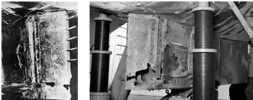
Figure 3. Damaged X-15-2 pylon from Mach 6.7 shock interference heating.
